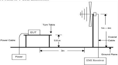
The diagram below shows the test setup that is utilized to make the measurements for emission from 1 GHz to 18 GHz Emissions.
