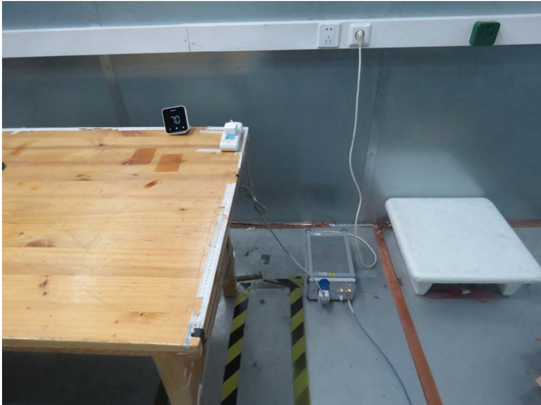
Picture 3 Conducted Emission Test Setup
