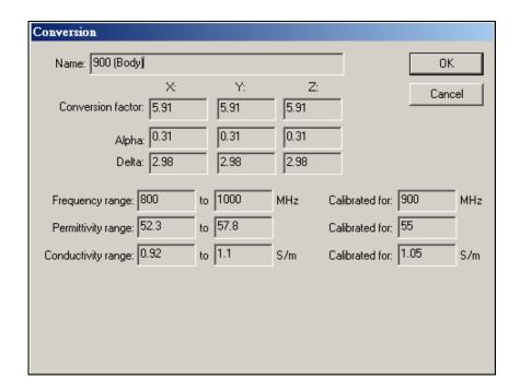
The target permittivity and conductivity at 835 MHz is 55.2 and 0.97 respectively which is within the calibrated range of the probe parameter.
