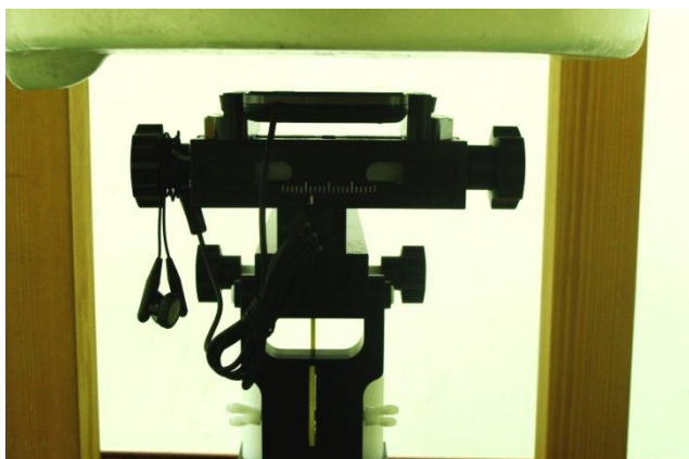
Face of the DUT with Phantom 1.5 cm Gap
