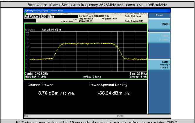
EUT stops transmission within 10 seconds of receiving instructions from its associated CBSD
