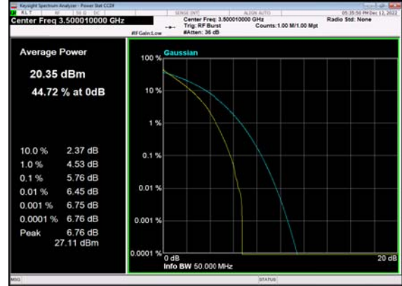
N77(50M)_DFT-s-OFDM QPSK Outer Full Mid CH
