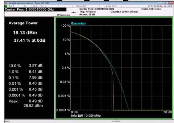
N77(10M)_CP-OFDM_16 QAM Outer Full Mid CH
