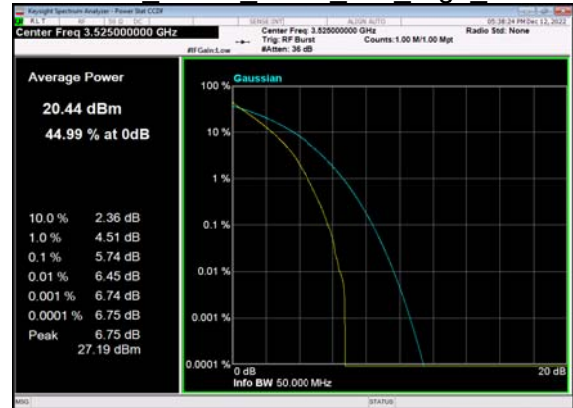
N77(50M)_DFT-s-OFDM QPSK Outer Full High CH
