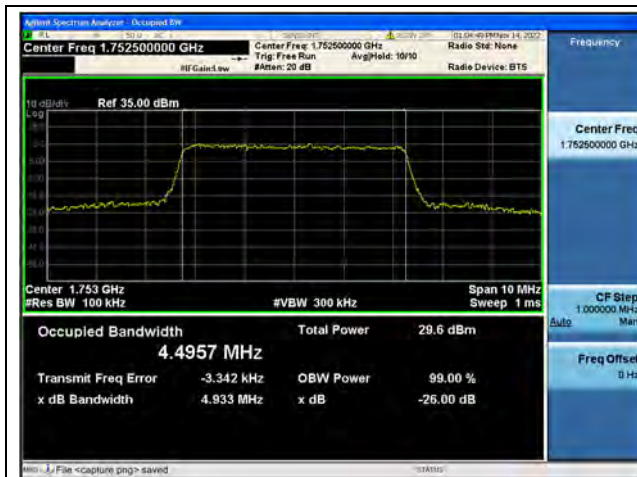
Band4 / 5MHz / QPSK/ High CH
