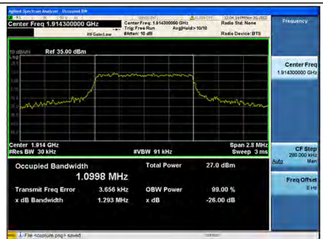
Band25 / 1.4MHz / 16QAM/ High CH
