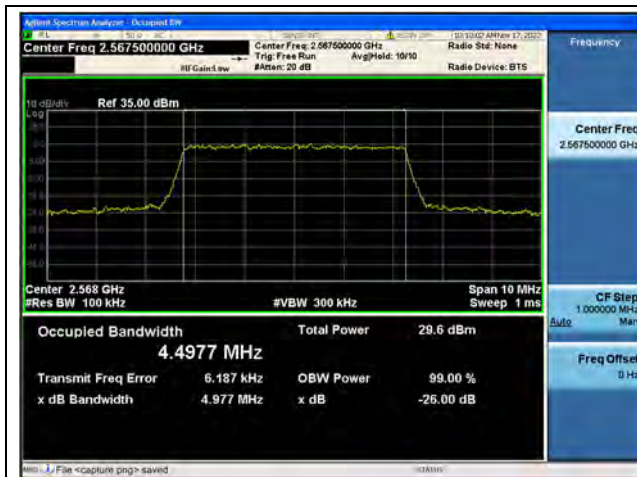
Band7 / 5MHz / QPSK/ High CH
