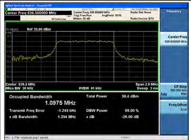
Band5 / 1.4MHz / QPSK/ Mid CH
