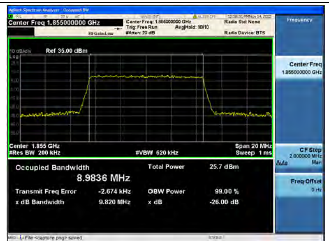
Band2 / 10MHz / 64QAM/ Low CH
