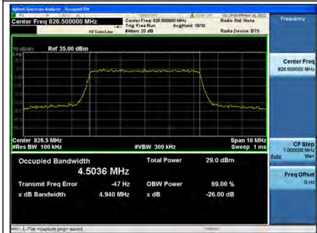
Band5 / 5MHz / 64QAM/ Low CH
