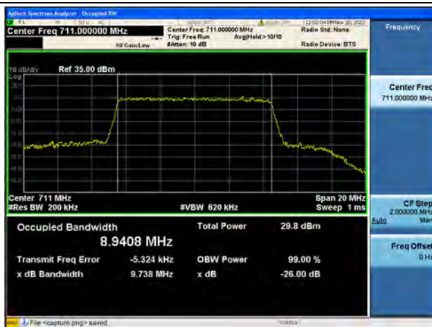
Band17 / 10MHz / 16QAM/ High CH
