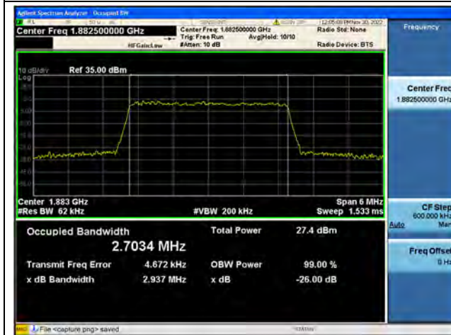
Band25 / 3MHz / 64QAM/ Mid CH
