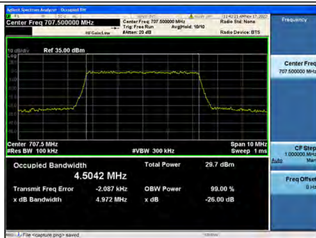
Band12 / 5MHz / 16QAM/ Mid CH
