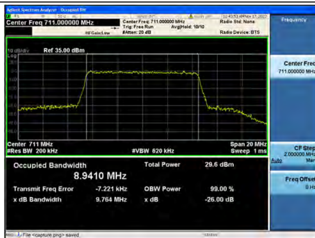
Band12 / 10MHz / 16QAM/ High CH
