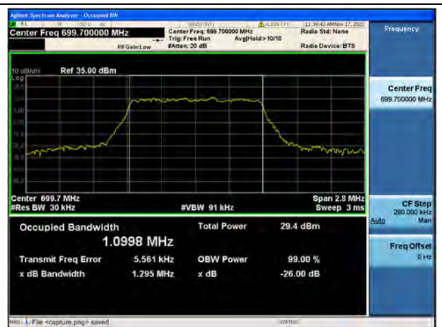
Band12 / 1.4MHz / 16QAM/ Low CH
