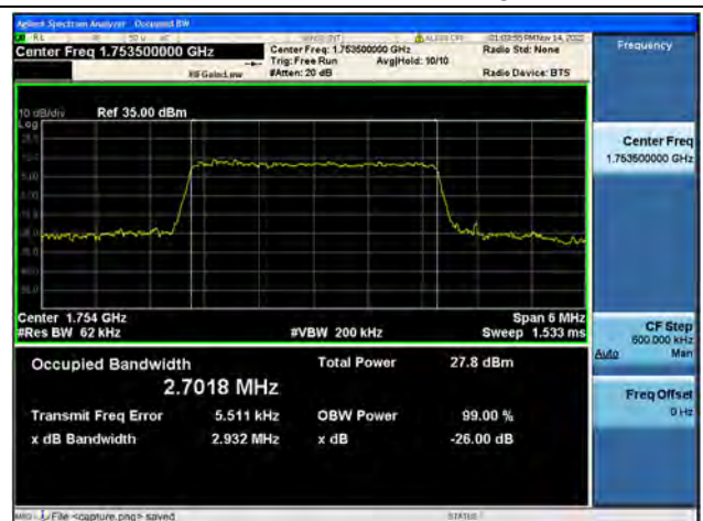
Band4 / 3MHz / 64QAM/ High CH
