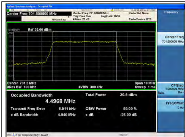
Band12 / 5MHz / QPSK/ Low CH
