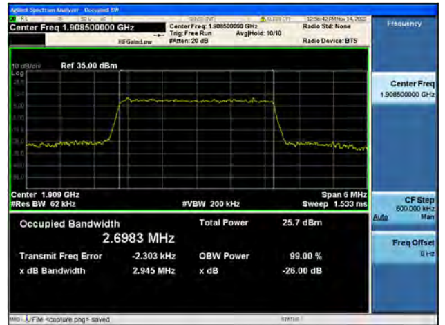
Band2 / 3MHz / QPSK/ High CH
