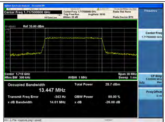
Band4 / 15MHz / 16QAM/ Low CH
