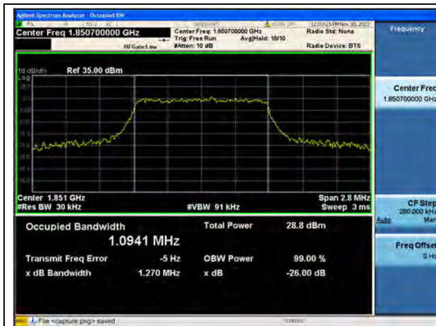
Band25 / 1.4MHz / QPSK/ Low CH
