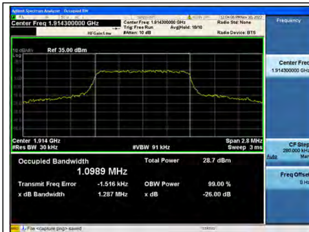
Band25 / 1.4MHz / QPSK/ High CH
