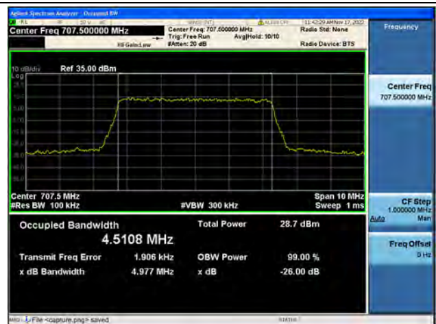
Band12 / 5MHz / 64QAM/ Mid CH
