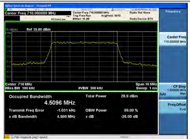
Band17 / 5MHz / 64QAM/ Mid CH
