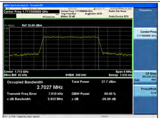
Band4 / 3MHz / 64QAM/ Low CH
