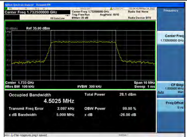
Band4 / 5MHz / 64QAM/ Mid CH
