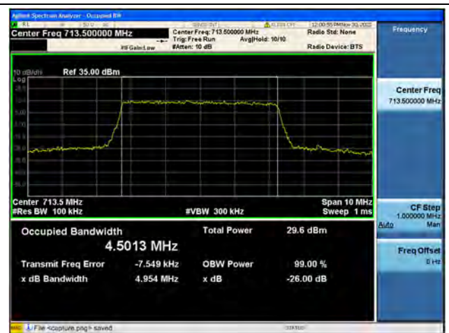
Band17 / 5MHz / 16QAM/ High CH
