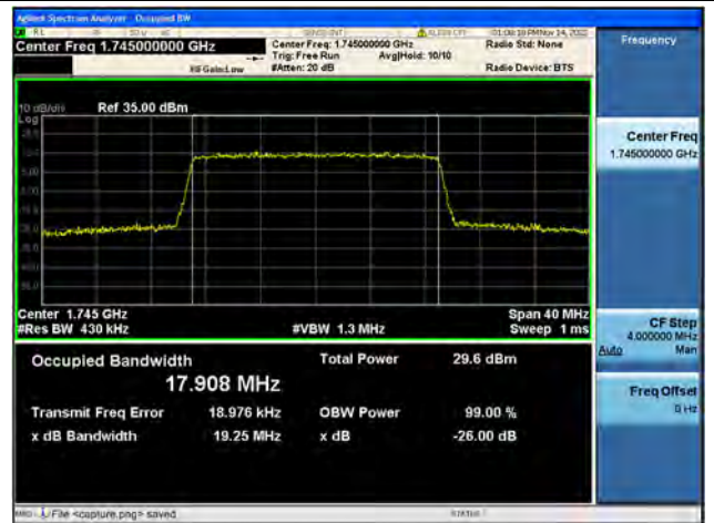
Band4 / 20MHz / QPSK/ High CH
