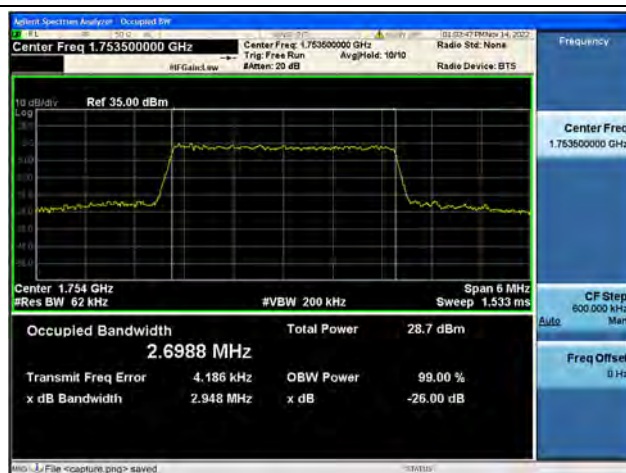
Band4 / 3MHz / 16QAM/ High CH
