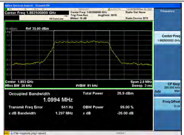
Band25 / 1.4MHz / 64QAM/ Mid CH
