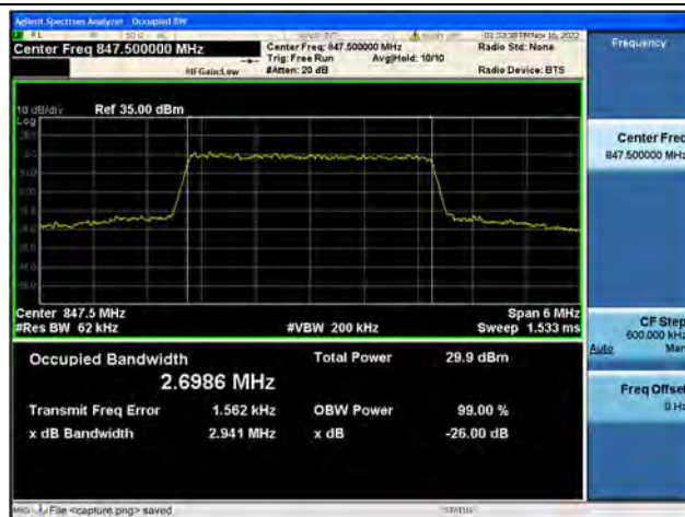
Band5 / 3MHz / 16QAM/ High CH
