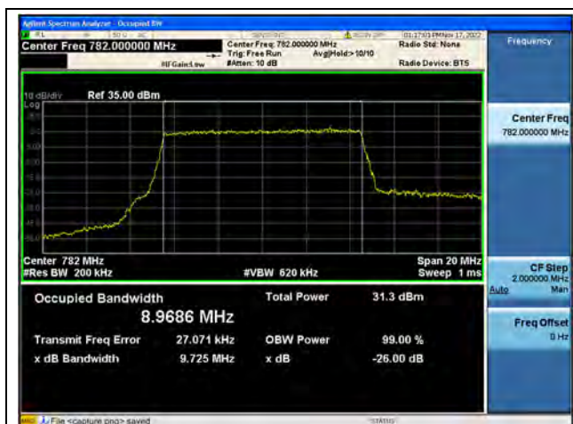
Band13 / 10MHz / QPSK/ Mid CH
