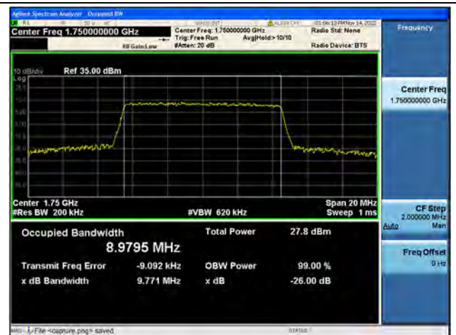
Band4 / 10MHz / 64QAM/ High CH
