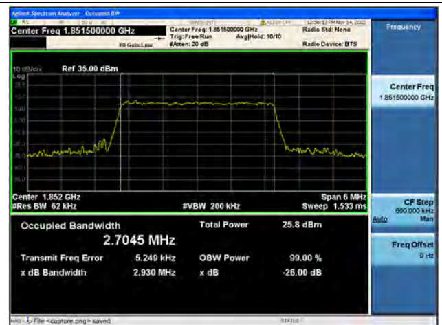
Band2 / 3MHz / 64QAM/ Low CH
