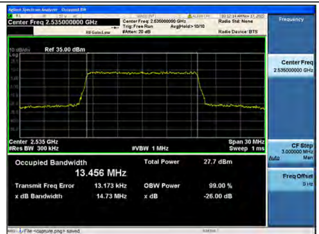
Band7 / 15MHz / 64QAM/ Mid CH
