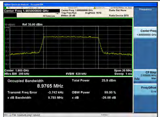
Band2 / 10MHz / QPSK/ High CH
