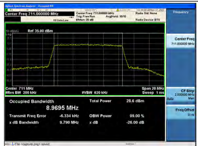
Band12 / 10MHz / 64QAM/ High CH
