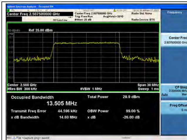
Band7 / 15MHz / QPSK/ Low CH
