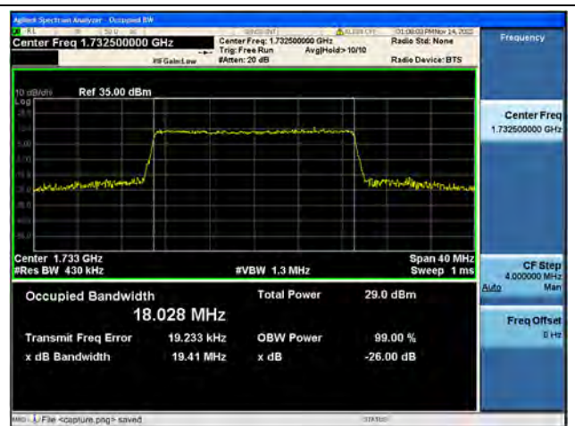
Band4 / 20MHz / 16QAM/ Mid CH
