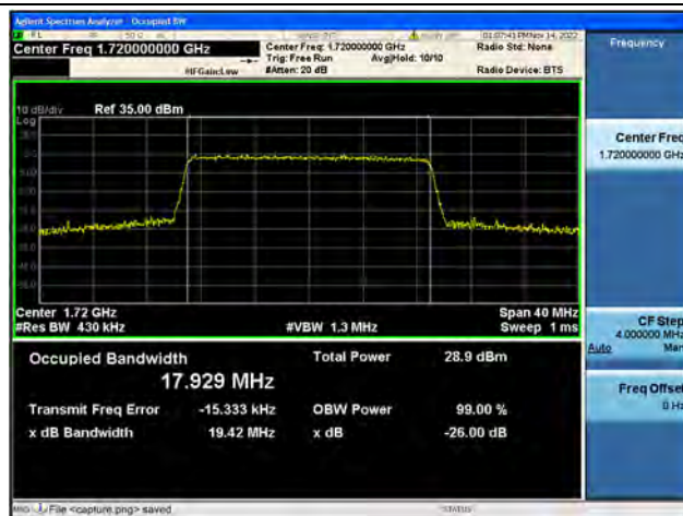
Band4 / 20MHz / 16QAM/ Low CH
