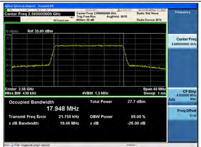
Band7 / 20MHz / 64QAM/ High CH
