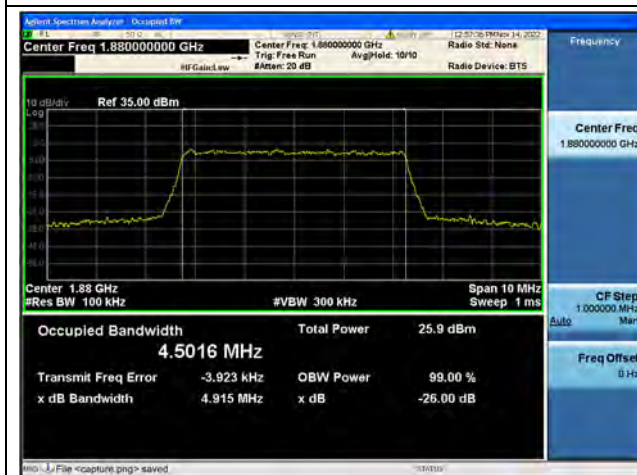
Band2 / 5MHz / 16QAM/ Mid CH
