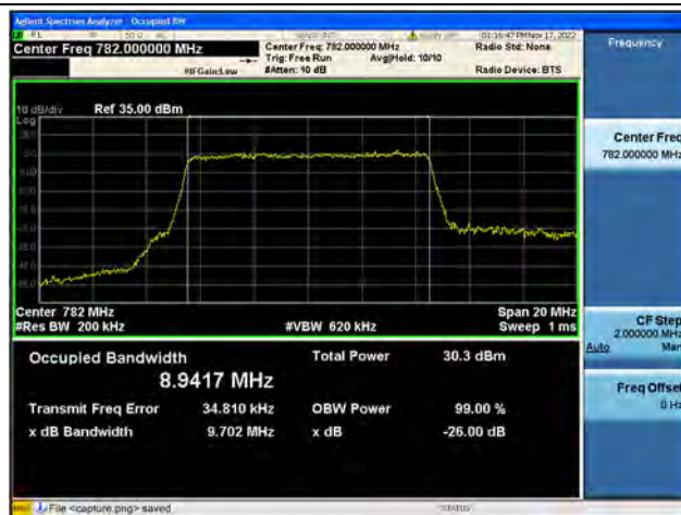
Band13 / 10MHz / 16QAM/ Low CH
