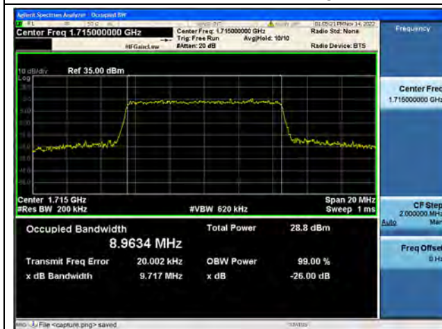
Band4 / 10MHz / 16QAM/ Low CH
