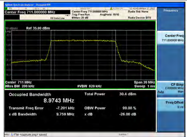
Band12 / 10MHz / QPSK/ High CH
