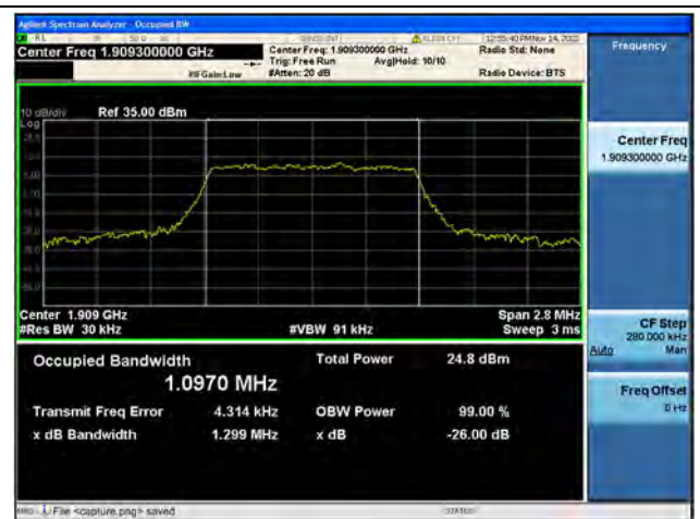
Band2 / 1.4MHz / 16QAM/ High CH
