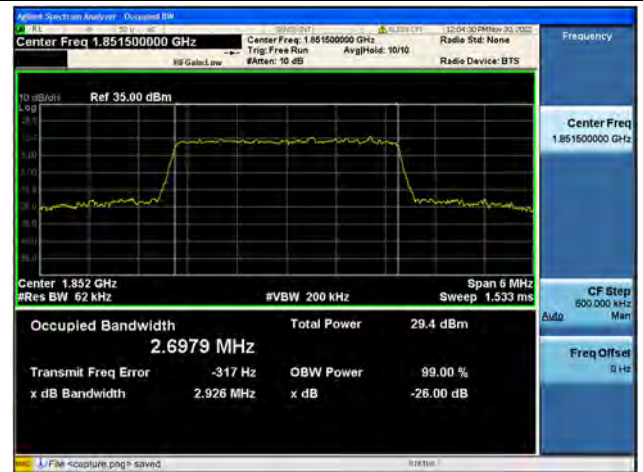
Band25 / 3MHz / QPSK/ Low CH
