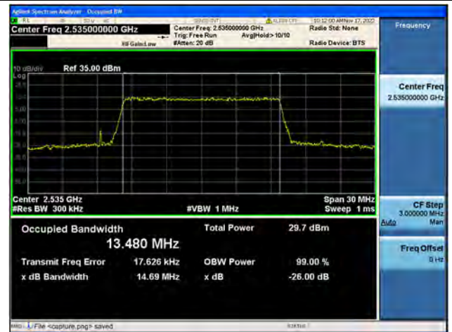
Band7 / 15MHz / QPSK/ Mid CH
