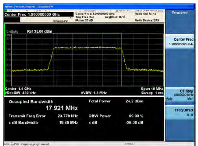
Band2 / 20MHz / 64QAM/ High CH
