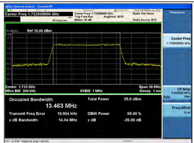
Band4 / 15MHz / 64QAM/ Mid CH
