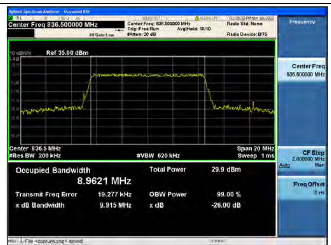
Band5 / 10MHz / 16QAM/ Mid CH
