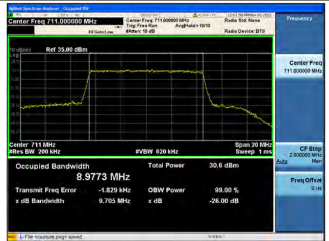
Band17 / 10MHz / QPSK/ High CH
