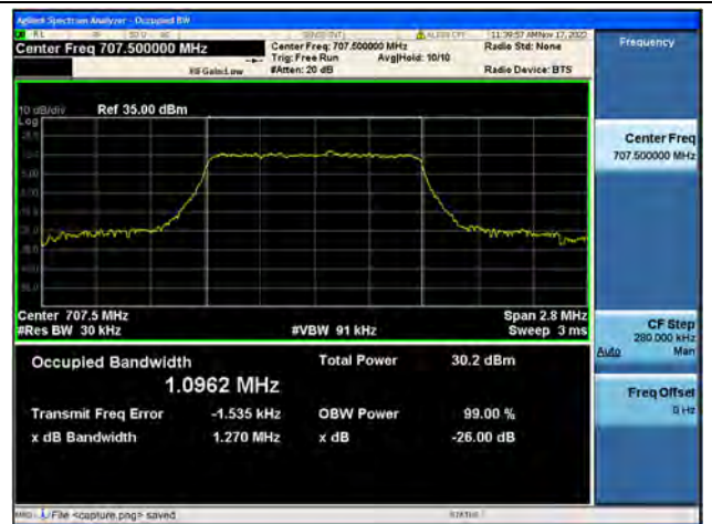
Band12 / 1.4MHz / QPSK/ Mid CH
