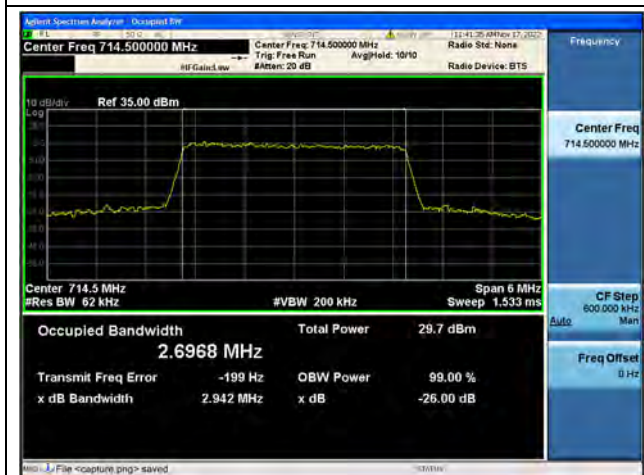
Band12 / 3MHz / 16QAM/ High CH
