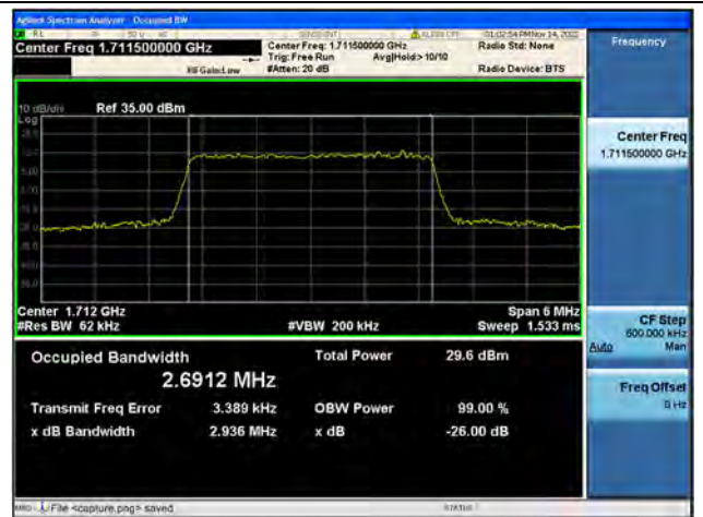
Band4 / 3MHz / QPSK/ Low CH
