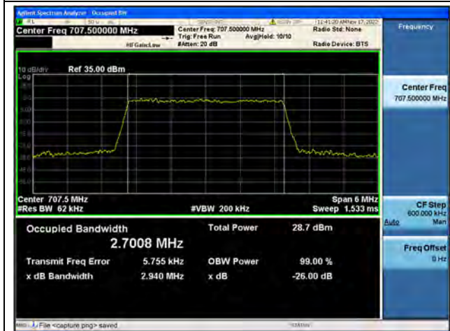
Band12 / 3MHz / 64QAM/ Mid CH
