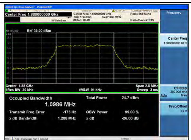
Band2 / 1.4MHz / 64QAM/ Mid CH
