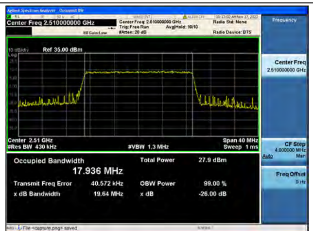
Band7 / 20MHz / 64QAM/ Low CH
