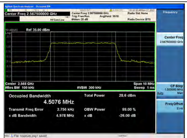
Band7 / 5MHz / 16QAM/ High CH
