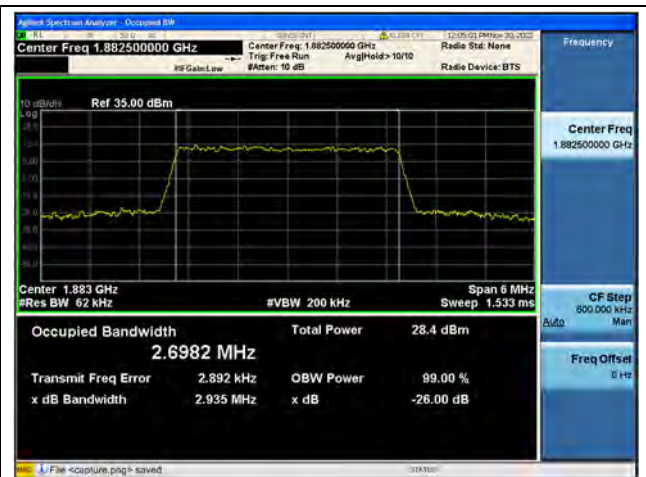
Band25 / 3MHz / 16QAM/ Mid CH
