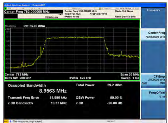
Band13 / 10MHz / 64QAM/ Low CH
