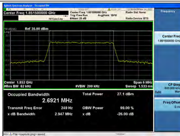
Band2 / 3MHz / 16QAM/ Low CH
