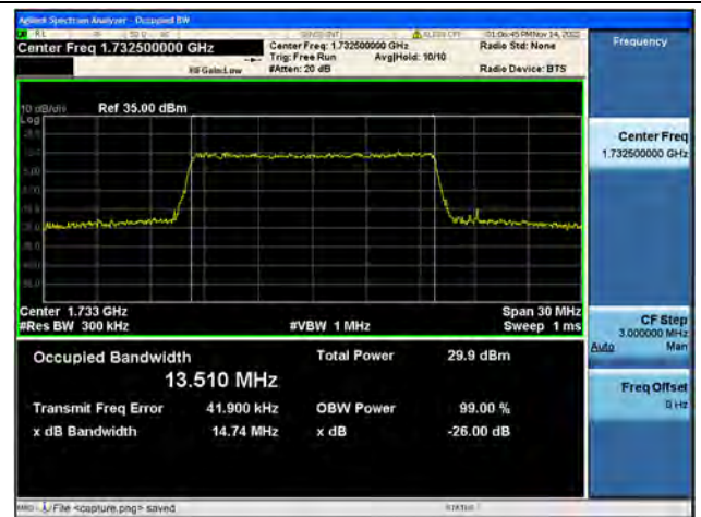
Band4 / 15MHz / QPSK/ Mid CH
