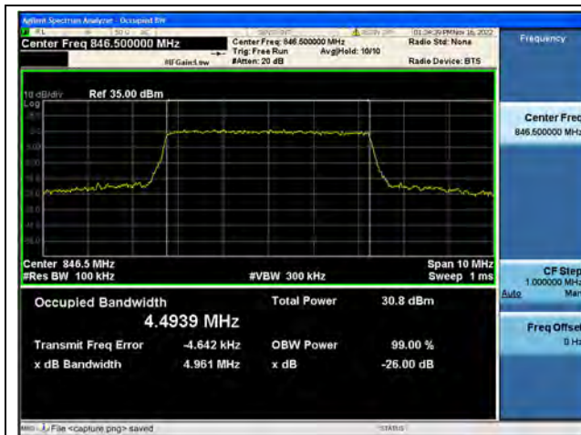
Band5 / 5MHz / QPSK/ High CH
