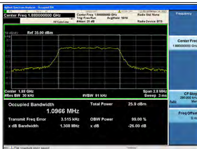
Band2 / 1.4MHz / 16QAM/ Mid CH
