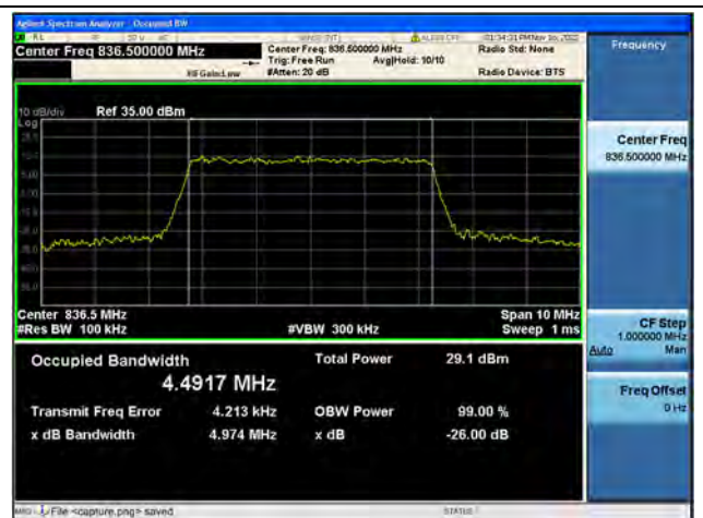
Band5 / 5MHz / 64QAM/ Mid CH
