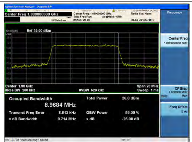
Band2 / 10MHz / 16QAM/ Mid CH
