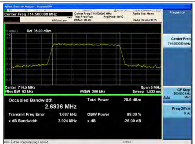
Band12 / 3MHz / 64QAM/ High CH
