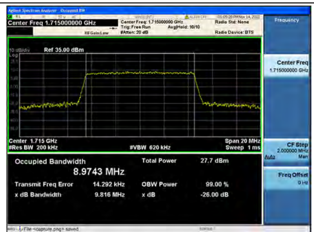
Band4 / 10MHz / 64QAM/ Low CH
