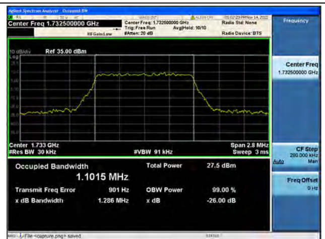
Band4 / 1.4MHz / 64QAM/ Mid CH
