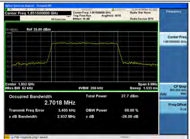
Band25 / 3MHz / 64QAM/ Low CH
