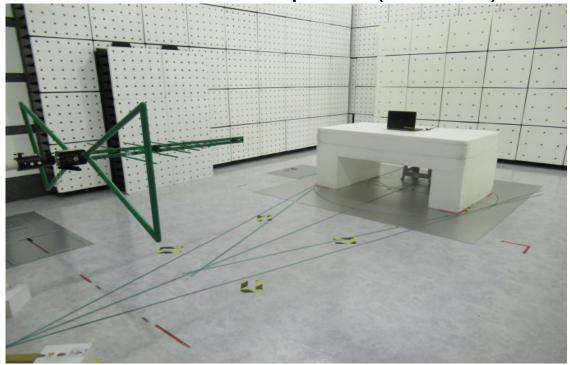
Radiated Emission Set up Photos (Above 1GHz)
