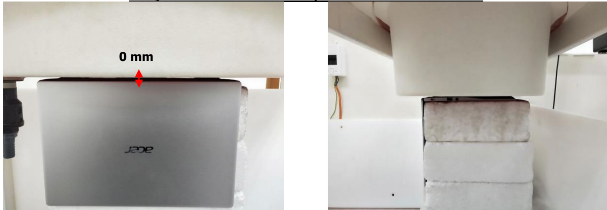
Fig.3 EUT Bottom side to flat phantom
