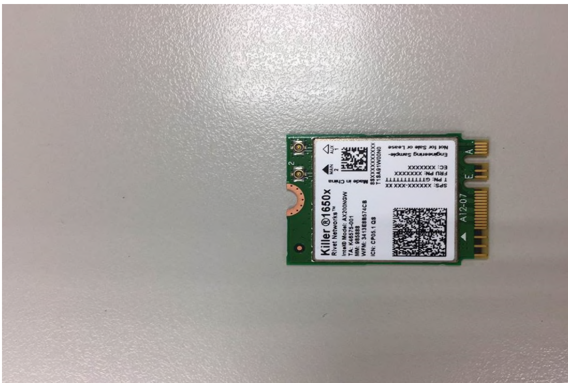
WLAN / BT Module - 1 (Model No.: AX200NGW)
