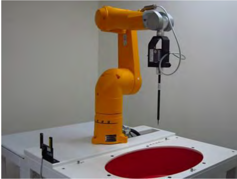
Fig.1 Photograph of the SAR measurement system
