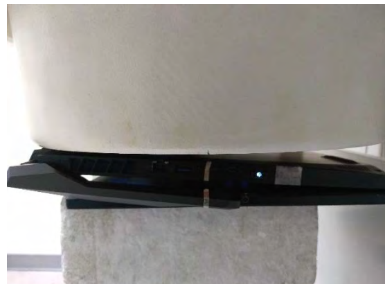
Fig.3 EUT Back side (Stand Mode) to flat phantom
