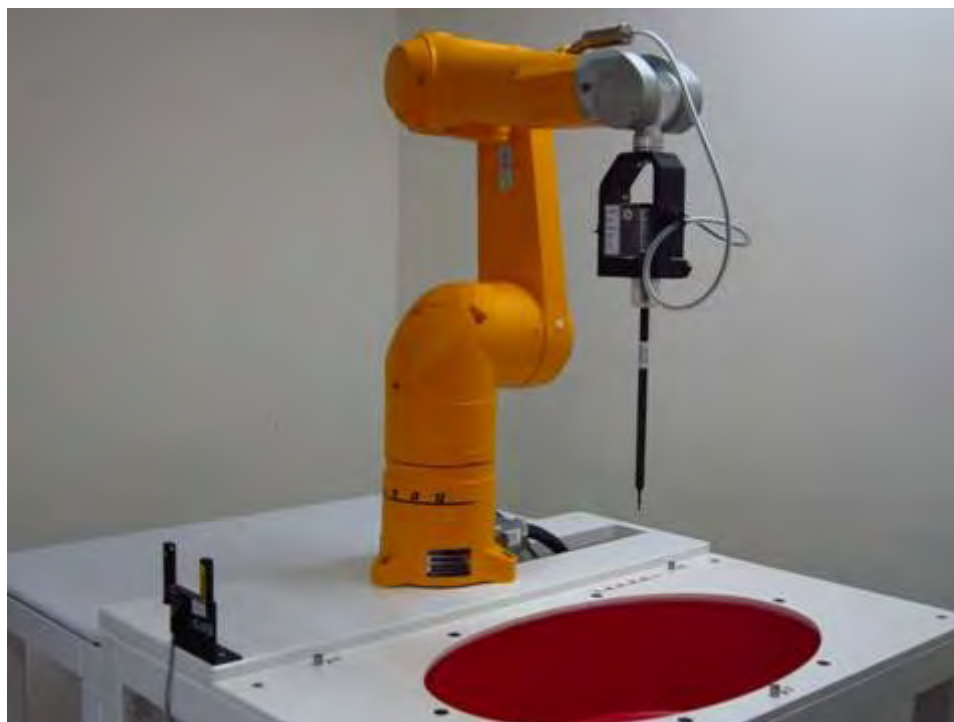
Fig.1 Photograph of the SAR measurement system
