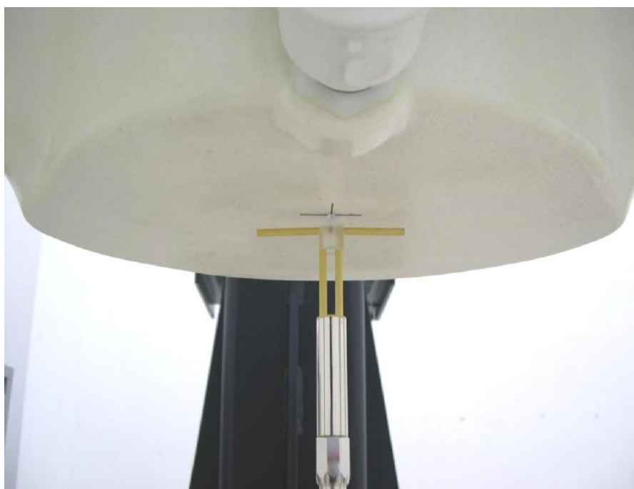
Picture 8.2 Photo of Dipole Setup
