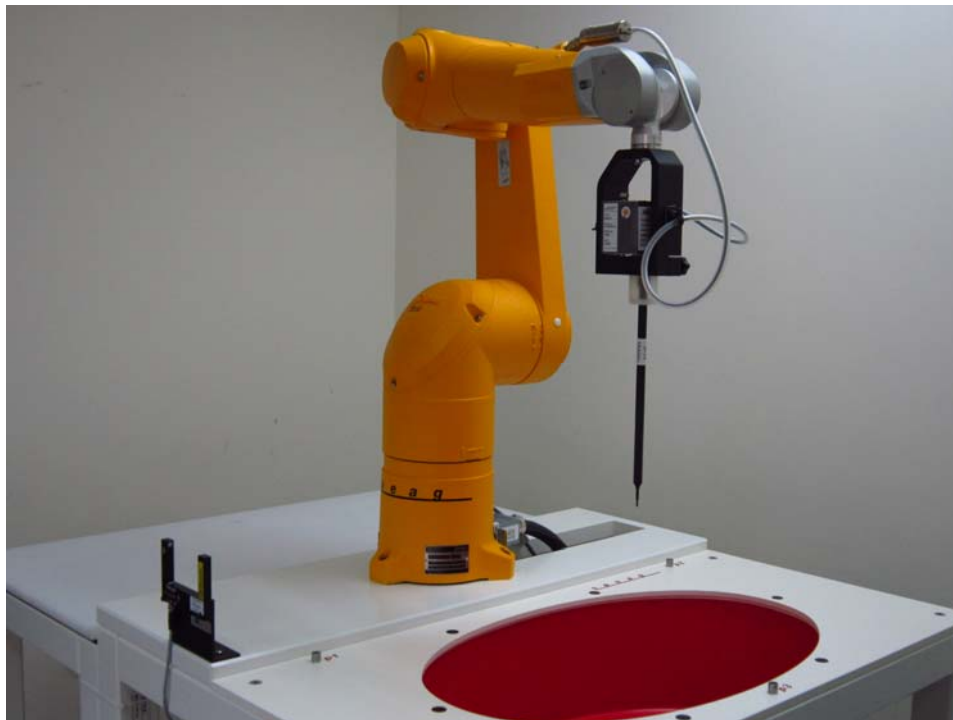
Fig.1 Photograph of the SAR measurement system
