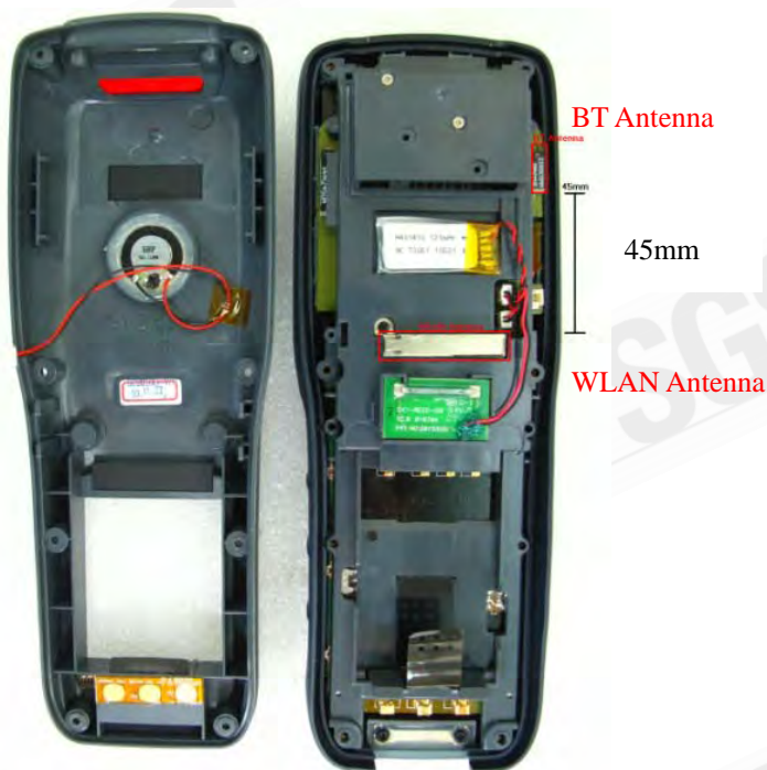
Fig.5 Antenna position & distance
