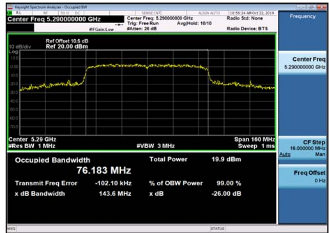
U-NII-2c 26dB Bandwidth-802.11n(20MHz ) ,5600MHz
