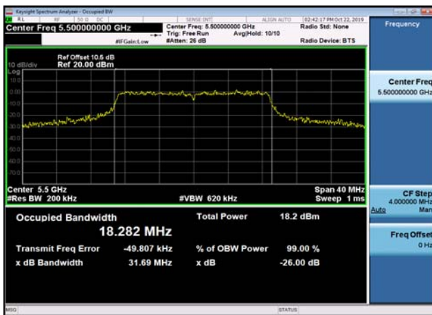
U-NII-2c 26dB Bandwidth-802.11n(20MHz ) ,5500MHz
