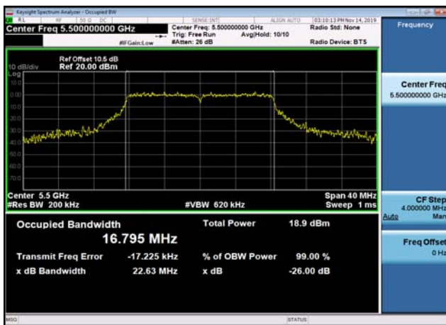
U-NII-2c 26dB Bandwidth-802.11a(20MHz )5500MHz
