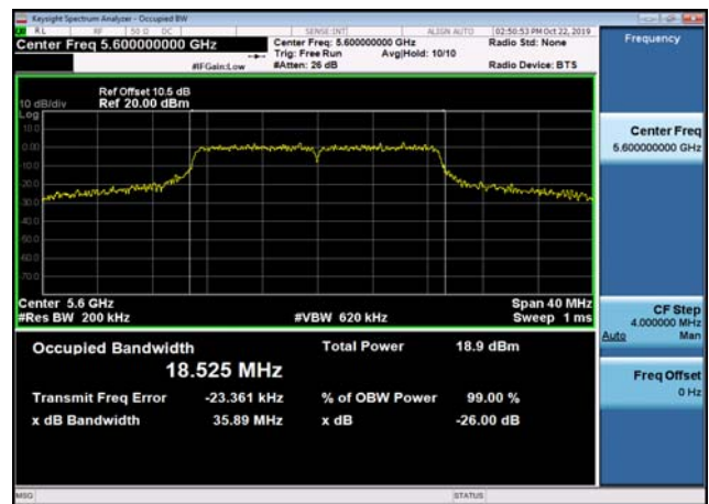
U-NII-2c 26dB Bandwidth-802.11n(20MHz ) ,5600MHz
