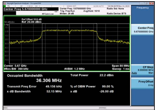
U-NII-2c 26dB Bandwidth-802.11a(20MHz )5600MHz
