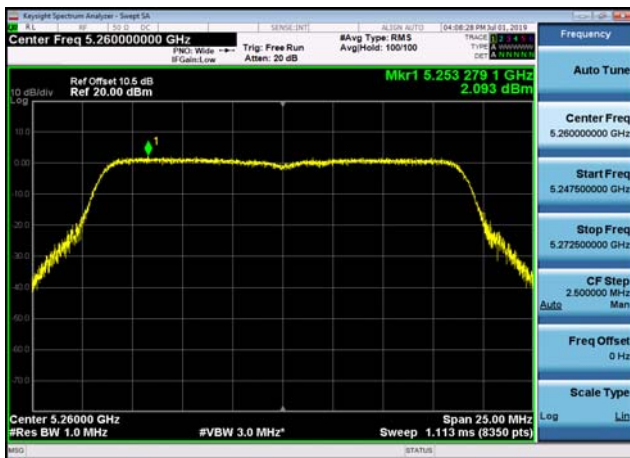
U-NII-2a Power spectral density-802.1 1ac(20MHz),5260MHz,Ant1
