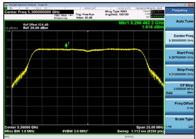
U-NII-2a Power spectral density-802.1 1ac(20MHz),5300MHz,Ant1
