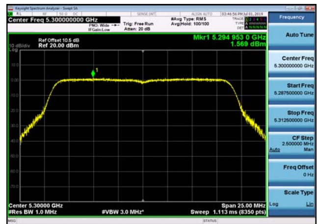
U-NII-2a Power spectral density-802.11 1n(40MHz),5270MHz,Ant1
