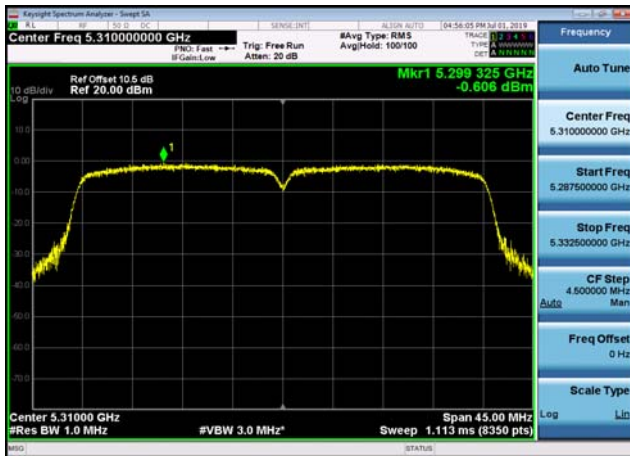
U-NII-2a Power spectral density-802.1 1a(20MHz),5300MHz,Ant1
