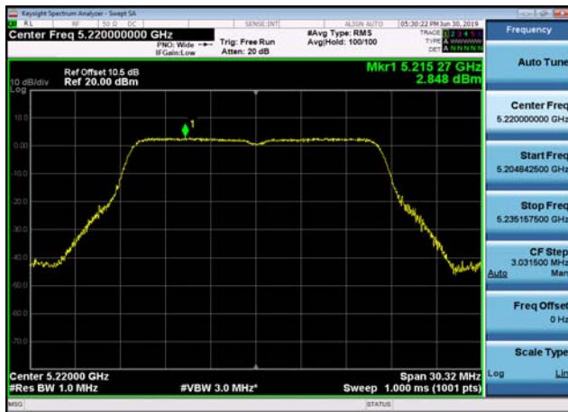
U-NII-1 Power spectral density-802.11 ac(20MHz),5180MHz,Ant1
