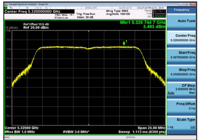
U-NII-2a Power spectral density-802.1 1ac(20MHz),5300MHz,Ant1
