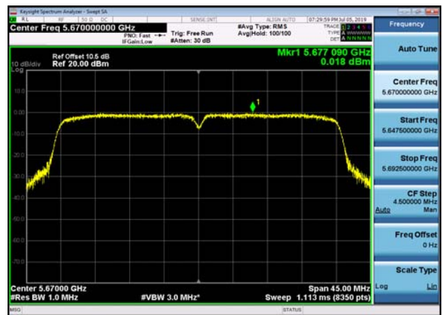
U-NII-2c Power spectral density-802.1 1a(20MHz),5600MHz,Ant1
