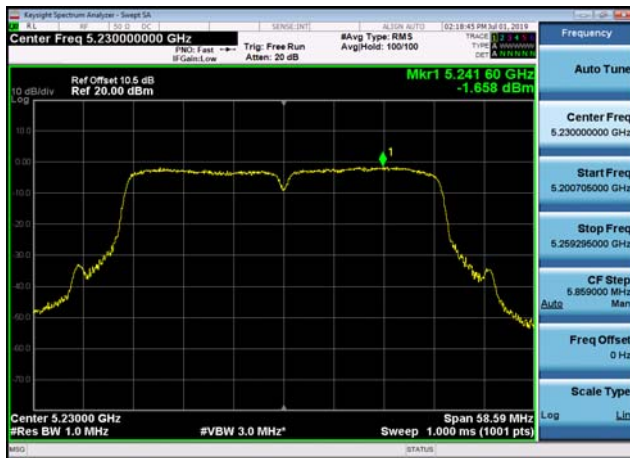
U-NII-2a Power spectral density-802.11 1n(20MHz),5260MHz,Ant1
