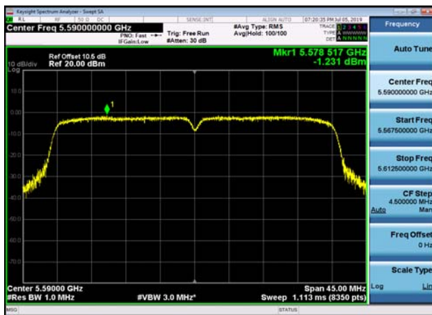
U-NII-2c Power spectral density-802.1 1a(20MHz),5500MHz,Ant1
