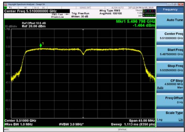
U-NII-2c Power spectral density-802.1 1n(40MHz),5670MHz,Ant1
