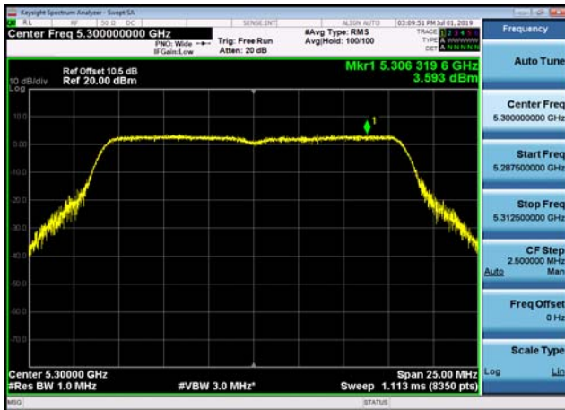
U-NII-2a Power spectral density-802.1 1ac(20MHz),5260MHz,Ant1
