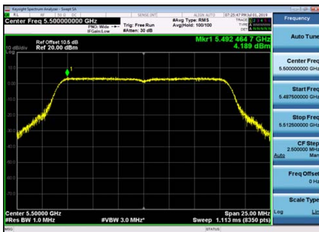
U-NII-2c Power spectral density-802.1 1a(20MHz),5500MHz,Ant1
