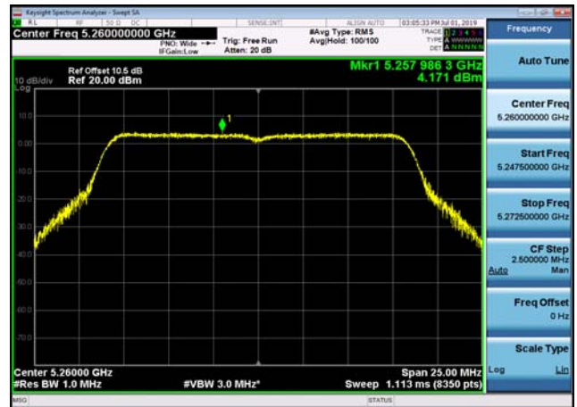
U-NII-2a Power spectral density-802.1 1a(20MHz),5320MHz,Ant1
