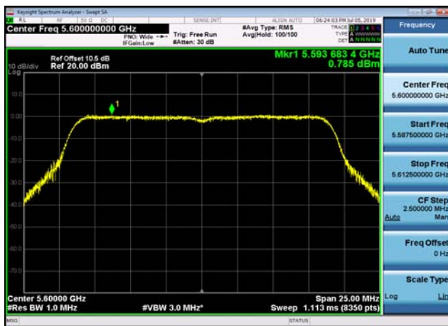
U-NII-2c Power spectral density-802.1 1ac(40MHz),5510MHz,Ant1
