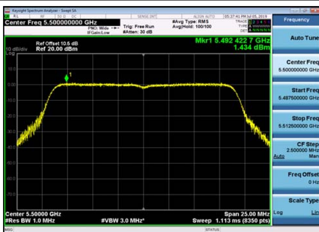
U-NII-2c Power spectral density-802.1 1n(20MHz),5500MHz,Ant1
