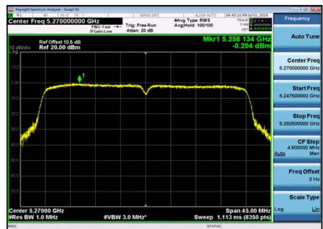
U-NII-2a Power spectral density-802.11 1n(40MHz),5270MHz,Ant1
