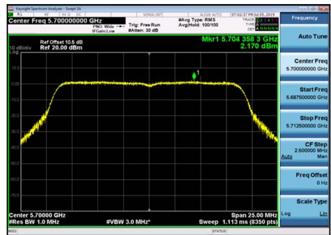
U-NII-2c Power spectral density-802.1 1ac(40MHz),5590MHz,Ant1
