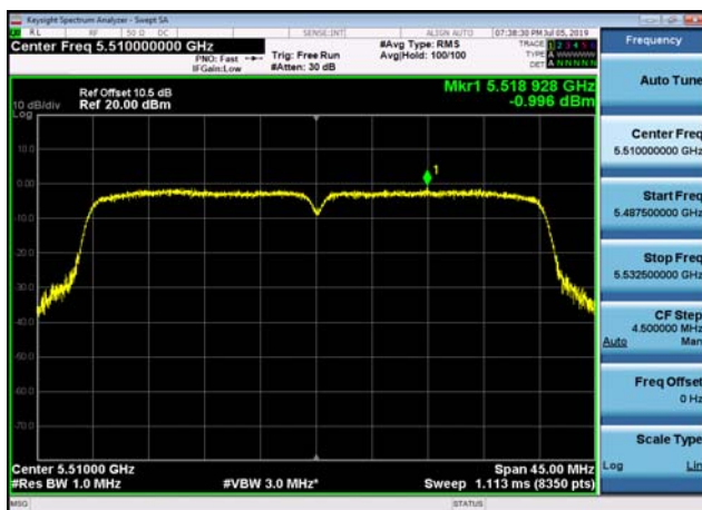
U-NII-2c Power spectral density-802.1 1ac(40MHz),5510MHz,Ant1
