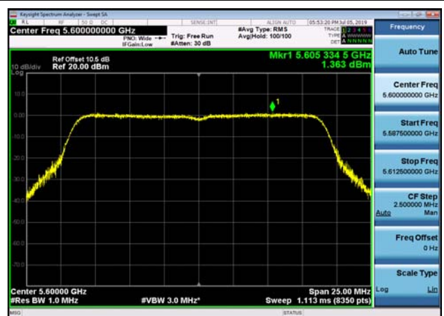
U-NII-2c Power spectral density-802.1 1n(20MHz),5600MHz,Ant1
