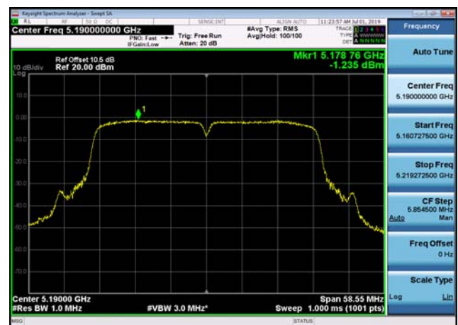
U-NII-1 Power spectral density-802.11 a(20MHz),5180MHz,Ant1
