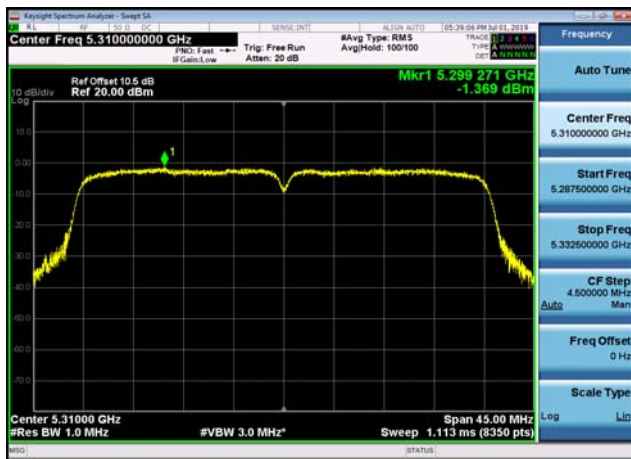
U-NII-2c Power spectral density-802.1 1n(20MHz),5500MHz,Ant1
