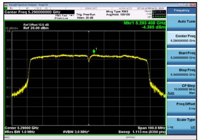
U-NII-2c Power spectral density-802.1 1n(20MHz),5600MHz,Ant1
