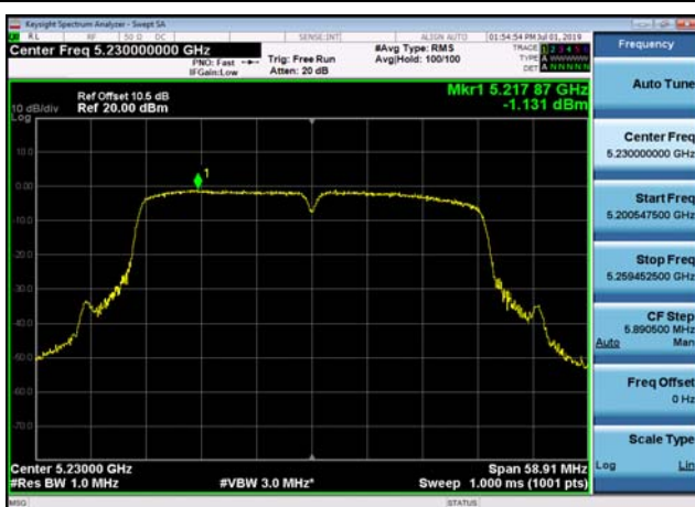
U-NII-1 Power spectral density-802.11 n(40MHz),5230MHz,Ant1
