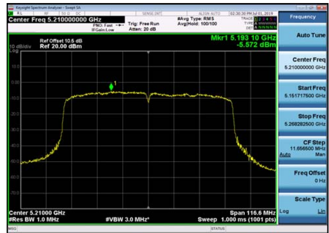
U-NII-2a Power spectral density-802.11 1n(20MHz),5300MHz,Ant1
