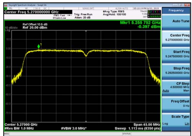
U-NII-2a Power spectral density-802.1 1ac(80MHz),5290MHz,Ant1
