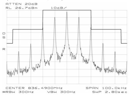
SAT + Voice; 836.49 MHz 100kHz Span, 300Hz RBW/VBW, Ref to power level
