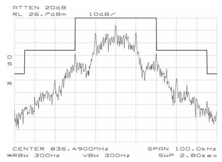
SAT; 836.49 MHz 100kHz Span, 300Hz RBW/VBW, Ref to power level
