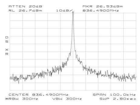
Voice; 836.49 MHz 100kHz Span, 300Hz RBW/VBW, Ref to power level
