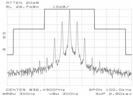
ST; 836.49 MHz 100kHz Span, 300Hz RBW/VBW, Ref to power level
