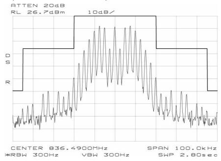
Wideband Data; 836.49 MHz 100kHz Span, 300Hz RBW/VBW, Ref to power level
