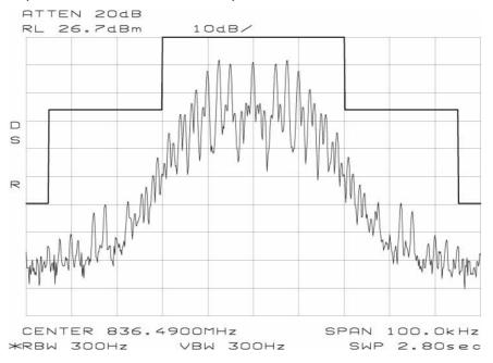
SAT + DTMF; 836.49 MHz 100kHz Span, 300Hz RBW/VBW, Ref to power level
