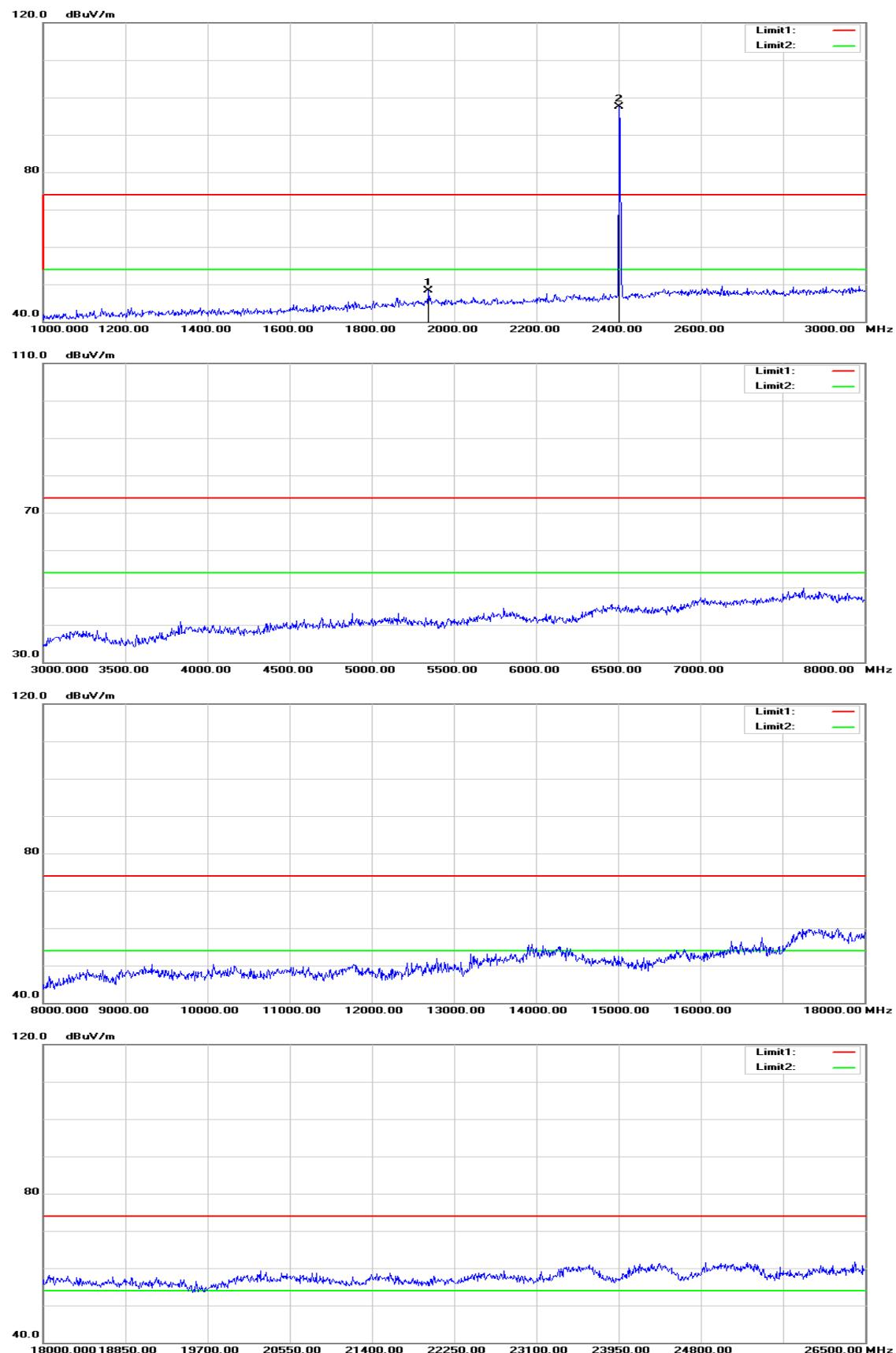
**Operation Mode:** GFSK / TX / CH Mid**Test Date:** January 10, 2016**Temperature:** 27°C**Tested by:** Jason Lu**Humidity:** 53 % RH**Polarity:** Ver. / Hor.
