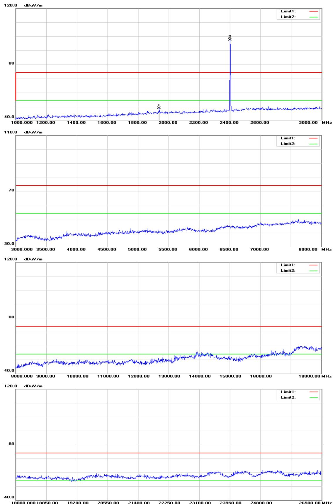
**Above 1 GHz****Operation Mode:** GFSK / TX / CH Low**Test Date:** January 10, 2016**Temperature:** 27°C**Tested by:** Jason Lu**Humidity:** 53 % RH**Polarity:** Ver. / Hor.
