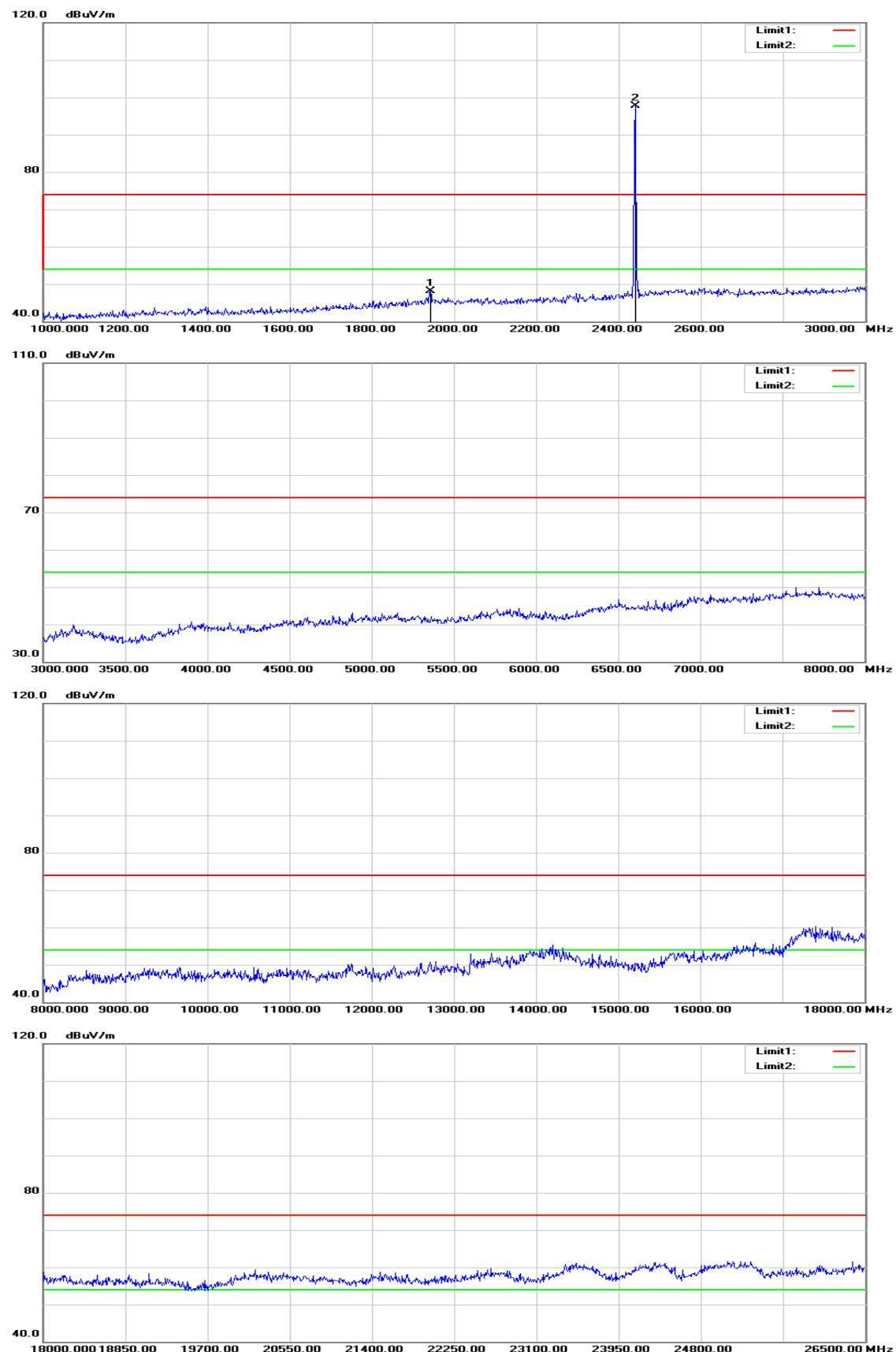
**Operation Mode:** GFSK / TX / CH High**Test Date:** January 10, 2016**Temperature:** 27°C**Tested by:** Jason Lu**Humidity:** 53 % RH**Polarity:** Ver. / Hor.
