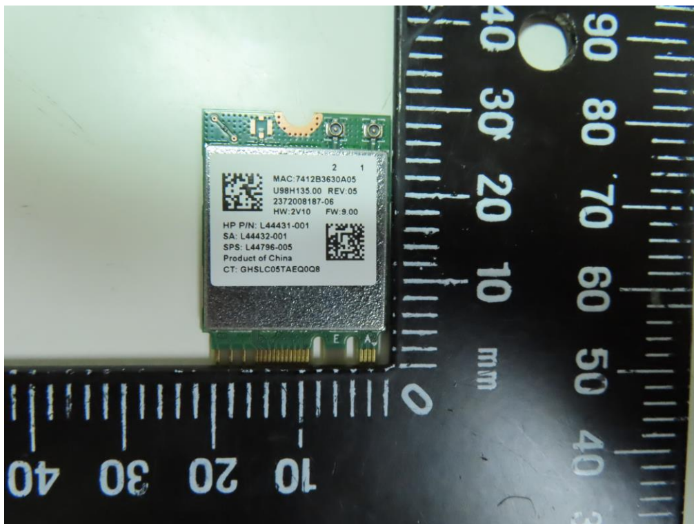
WLAN / BT Module -1 (Model No. : RTL8822CE)
