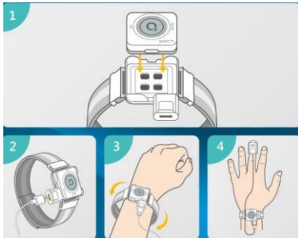
Step 1: Snap OQCA Pulse Oximeter onto the Holder.
