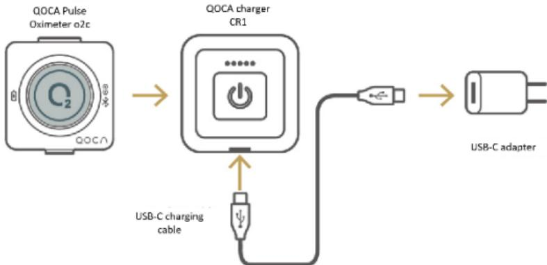
1. Use an AC adapter conforming to standard IEC 60601-1 與 IEC 62368-1 class II) with a USB-C interface to connect the charger or connect the charger to PC by the provided USB-C cable. **AC**
