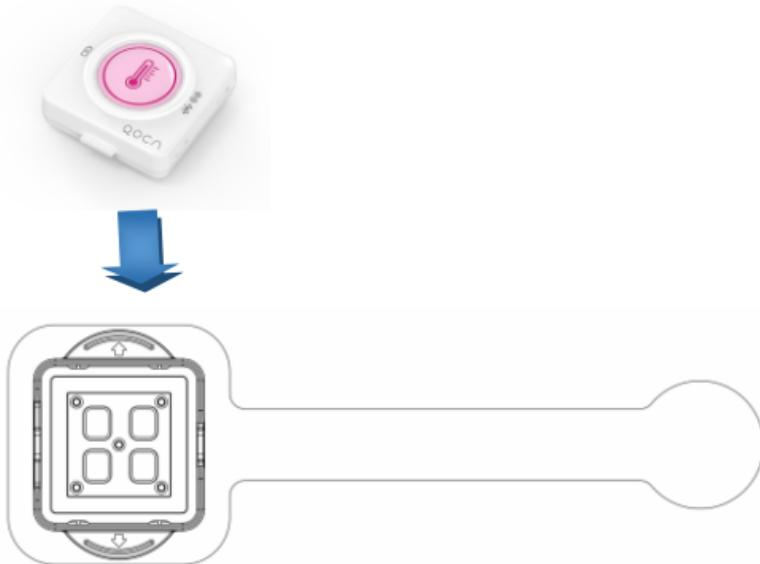
Step 2: Press the power button till QOCA Wearable BLE Thermometer flash green light\*\*. ( After power on, the status indicator “
