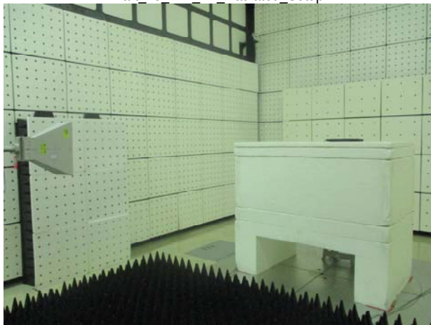
Part 15 247 LE Radiated Setup
