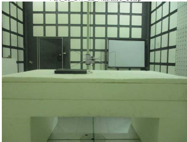
Part 15 247 LE Radiated Setup
