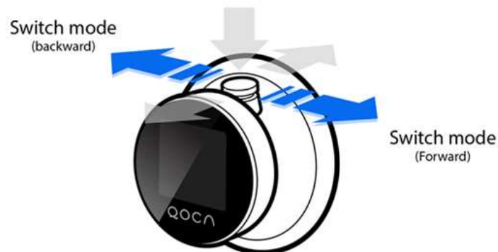
Fig16 、 The operation of joystick to switch mode
