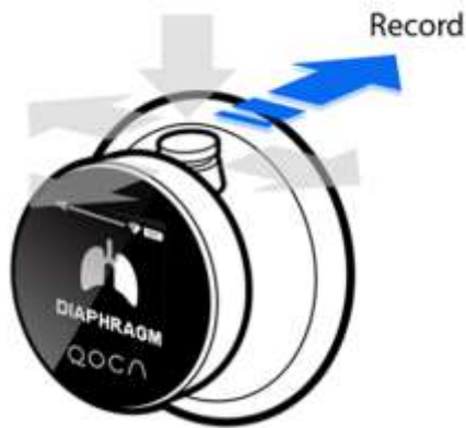
Fig13 、 The operation of joystick to enable record function
