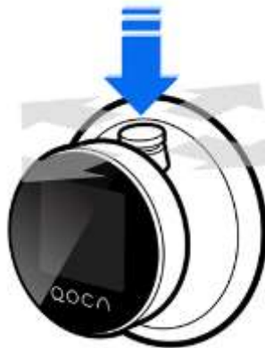
Fig5 、 The operation of joystick to enter pairing mode
