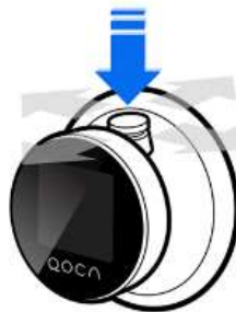
Fig8 、 Press the joystick to power on QOCA Wireless Digital Stethoscope
