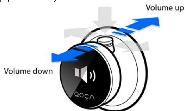
Fig18 、 The operation of joystick to adjust the volume
