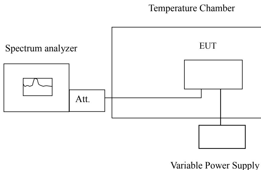
**Remark:** Measurement setup for testing on Antenna connector.
