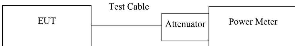
**Remark:** Measurement setup for testing on Antenna connector
