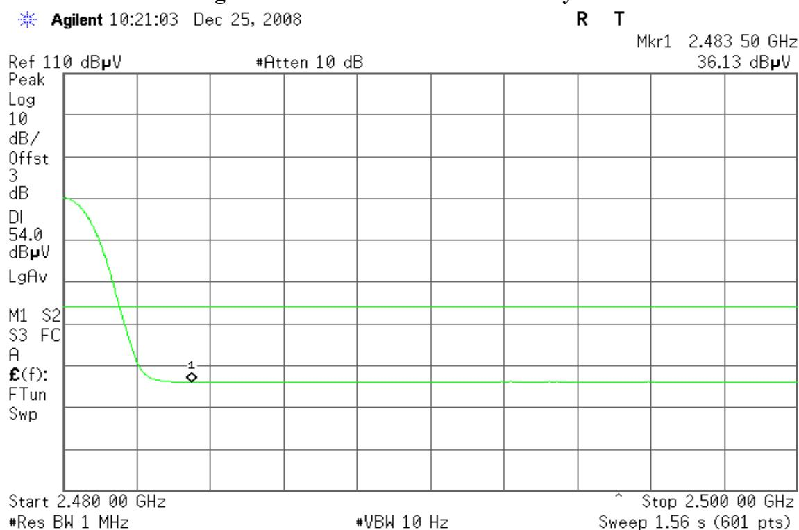
**For 8DPSK / DH5****Band Edges (CH Low)****Detector mode: Peak**
