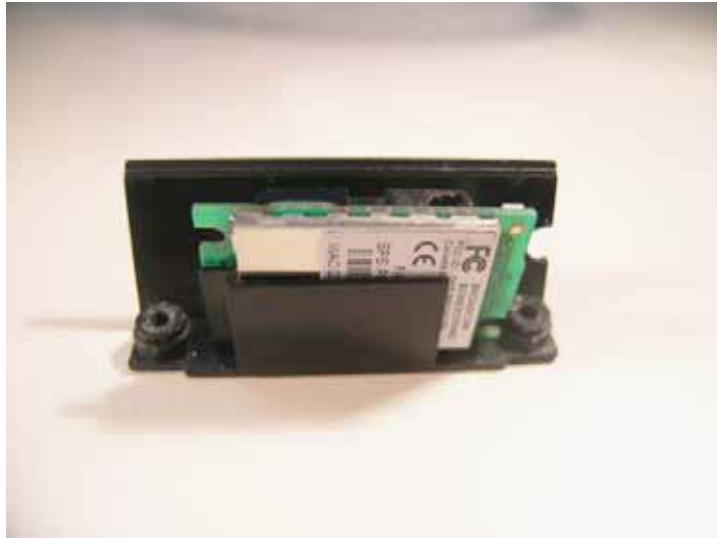
Antenna Module mounted in plastic Holder
