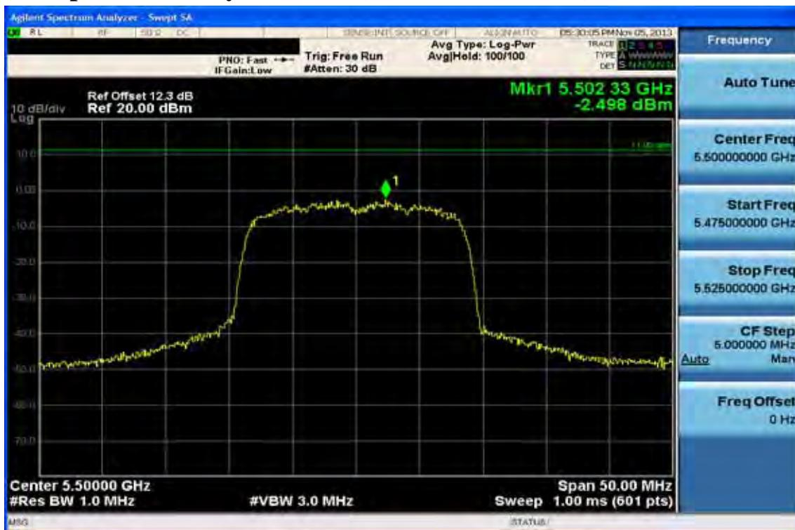
**Peak Power Spectral Density Data Plot (CH Mid 5580 MHz)**
