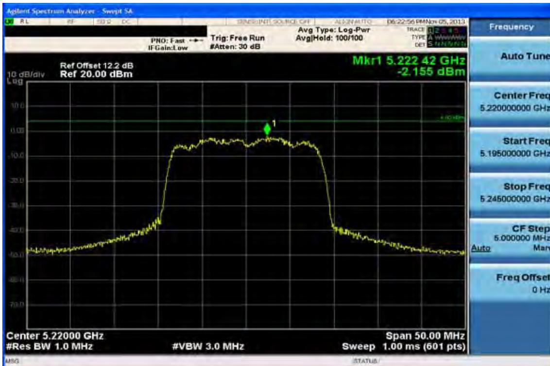
**802.11a, 5250~5350 MHz, PPSD Data Plot (CH Mid 5300 MHz)**
