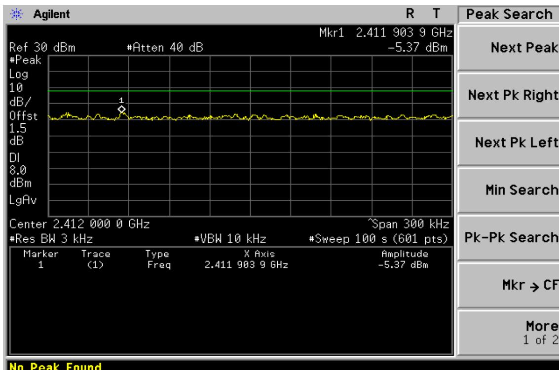
**Power Spectral Density Test Plot (CH-Mid)**
