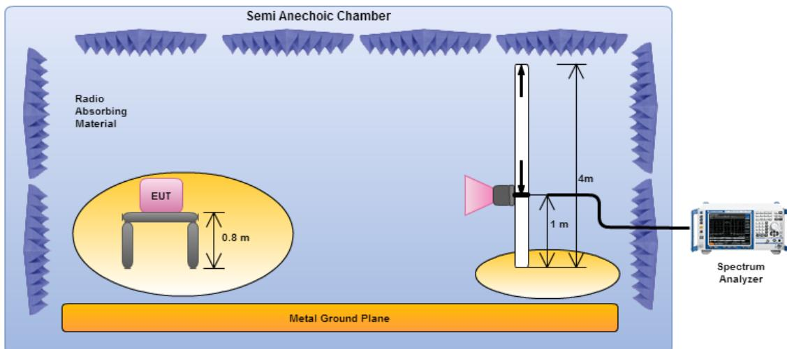
Magnetic field tests shall be performed in the frequency range of 9 kHz to 30 MHz using a calibrated loop antenna. Electric field tests shall be performed in the frequency range of 30 MHz to 1000 MHz using a calibrated bi-log antenna and the frequency range of 1 GHz to 40 GHz using a calibrated horn antenna.
