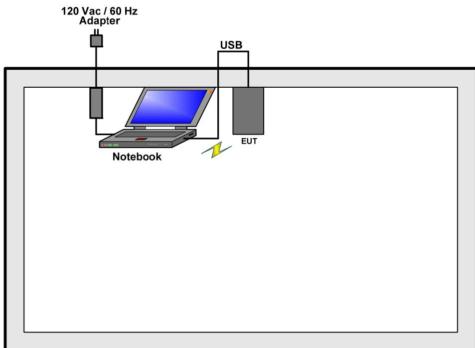
**Test Setup Diagram - Radiated Above 1GHz Test****Operating Mode 1 | AC Power & Continuous Transmitting**
