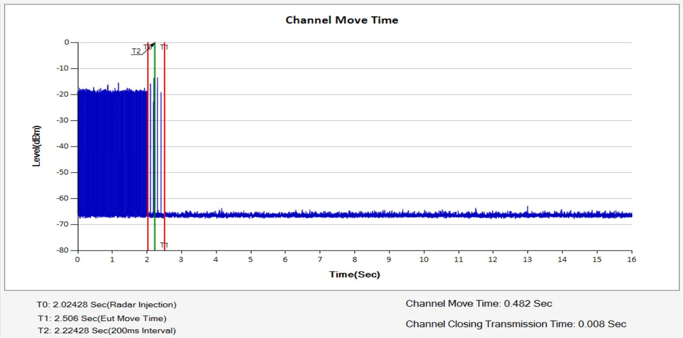
**Verdict:** Note: narrowing the sweep time as the good engineering process for the verification of transmission closing in 200ms
