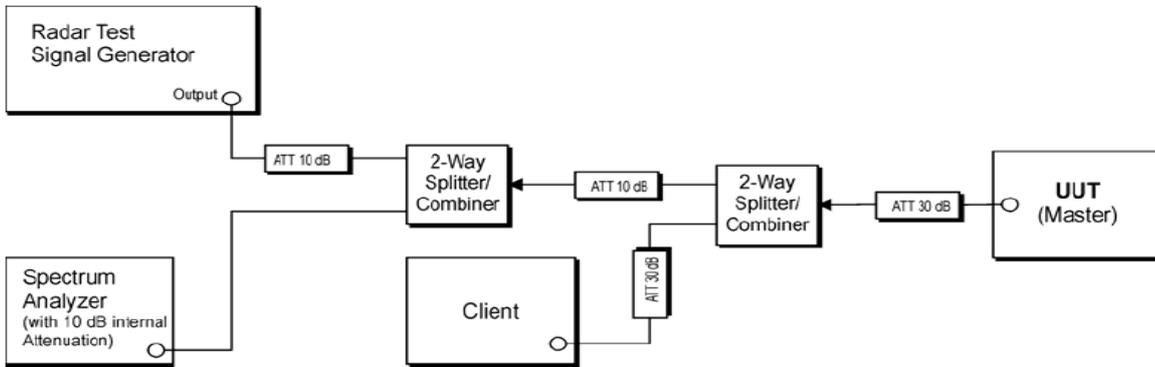
Setup for Client with injection at the Master
