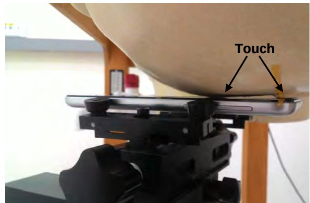
Fig.5 Left Head Section / Cheek-Touch Position
