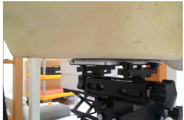
Fig.7 EUT Back side to flat phantom
