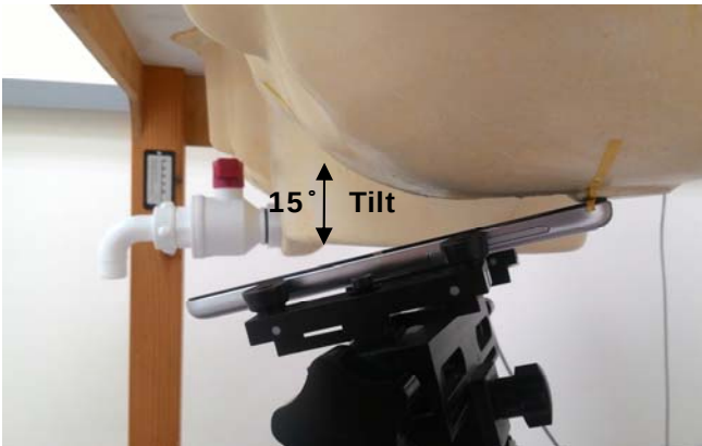
Fig.6 Left Head Section / Ear-Tilt Position(15°)
