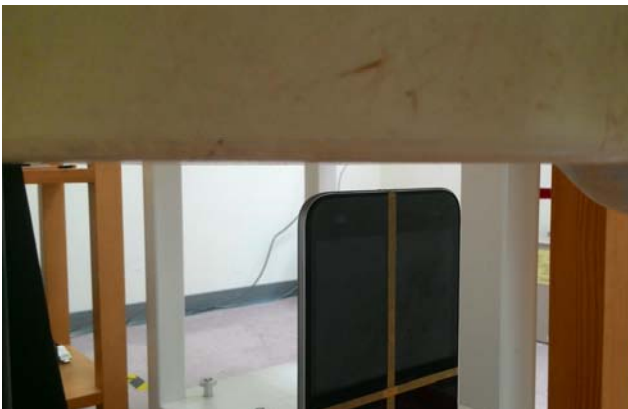
Fig.10 EUT bottom side to flat phantom
