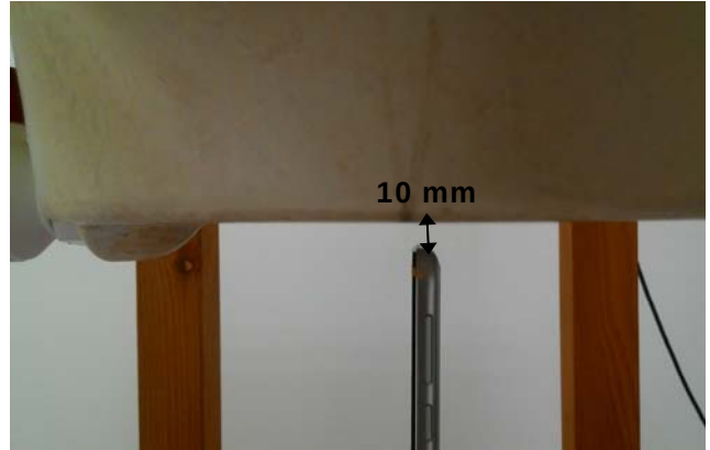
Fig.11 EUT top to flat phantom
