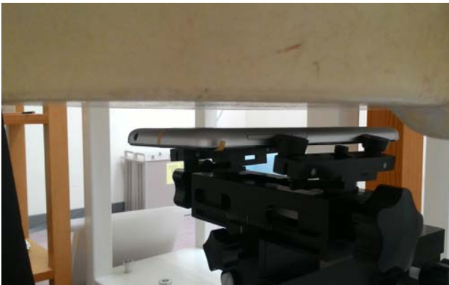
Fig.9 EUT back side to flat phantom
