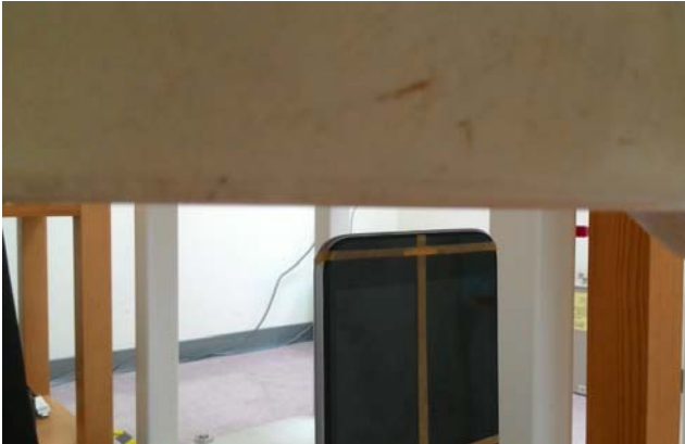
Fig.11 EUT top to flat phantom
