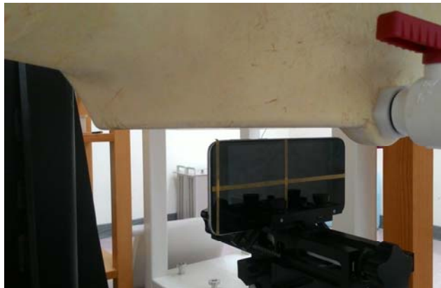
Fig.12 EUT right to flat phantom
