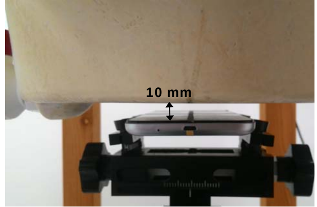
Fig.8 EUT front side to flat phantom
