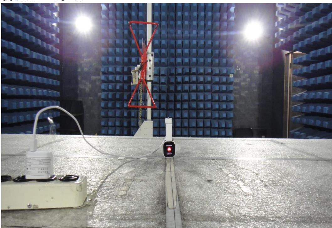
**Powerline Conducted Emissions Setup Photos**
