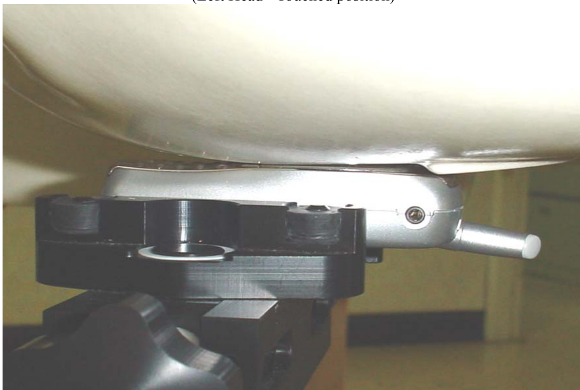
EUT Setup Configuration 2 (Left Head - Tilted position)
