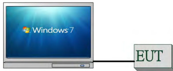
Fig. 2-2 Conducted Emission Configuration
