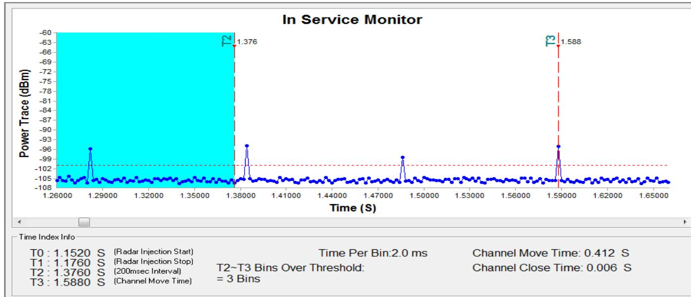
**Verdict:** Note: narrowing the sweep time as the good engineering process for the verification of transmission closing in 200ms
