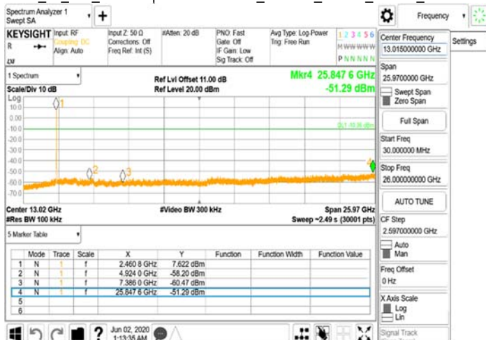
FCC 15 247 WLAN\Spurious Emission_802.11b_20MHz_Chain0_2462MHz
