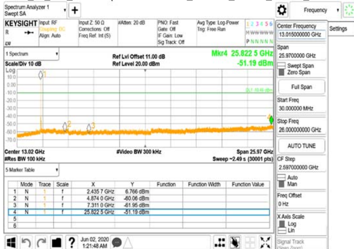
FCC 15 247 WLAN\Spurious Emission_802.11b_20MHz_Chain0_2462MHz
