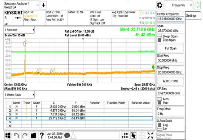
FCC 15 247 WLAN\Spurious Emission_802.11g_20MHz_Chain0_2462MHz
