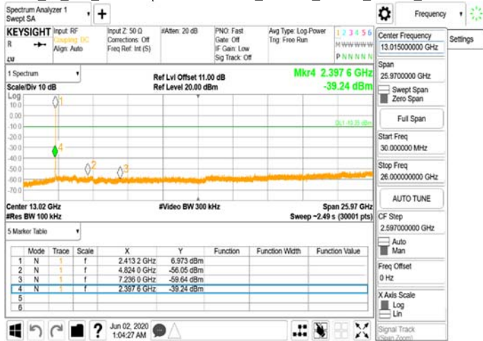
FCC 15 247 WLAN\Spurious Emission_802.11b_20MHz_Chain0_2437MHz
