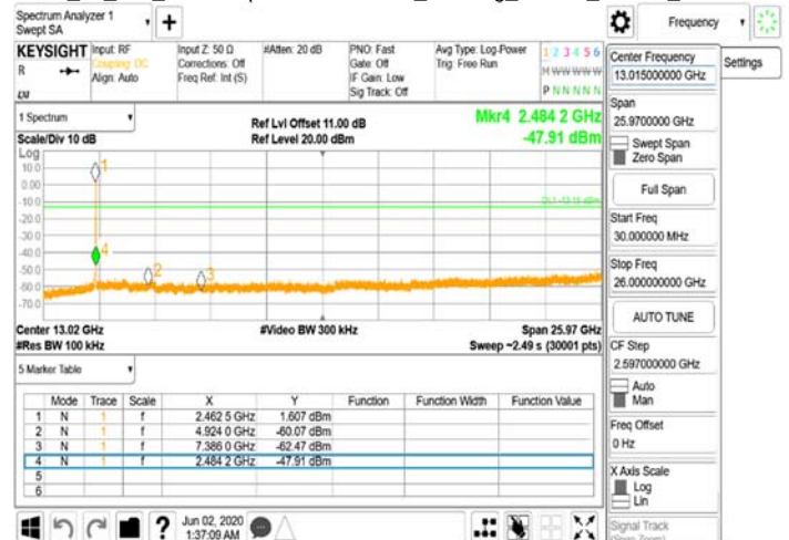
FCC 15 247 WLAN\Spurious Emission_802.11g_20MHz_Chain0_2462MHz
