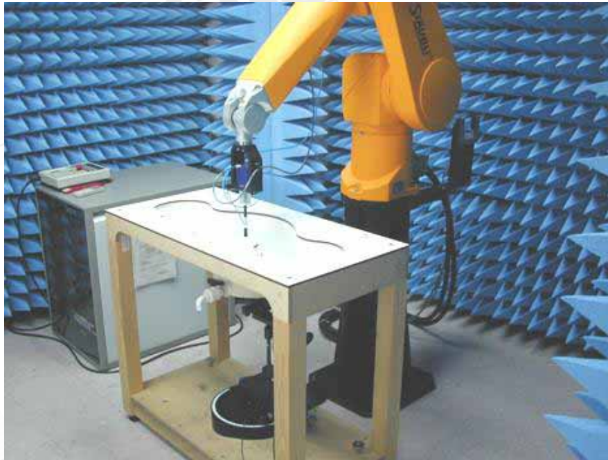
Fig.1 Photograph of the SAR measurement System
