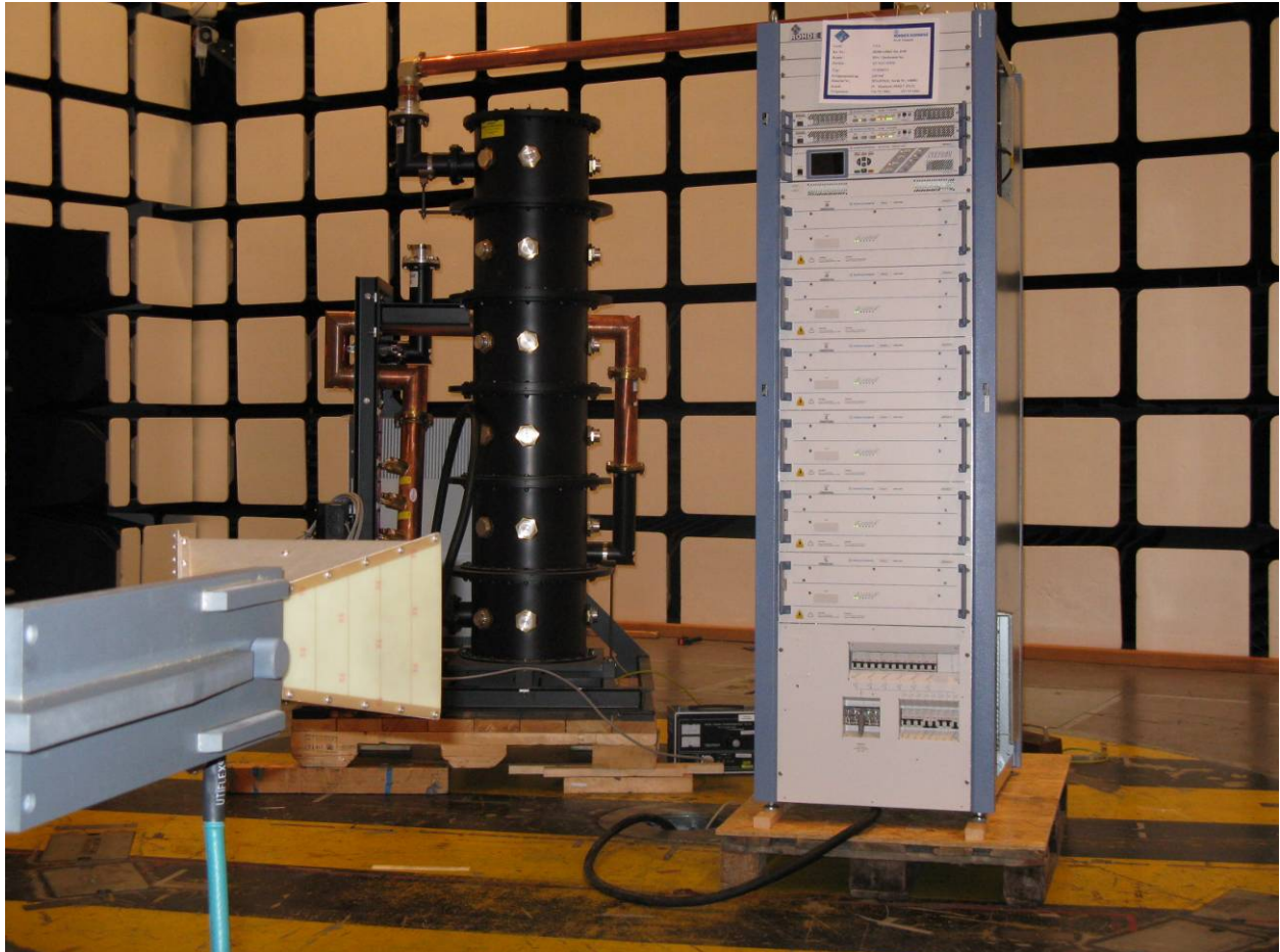
Figure 6-4: Test setup for radiated emission measurement, 1 - 10GHz
