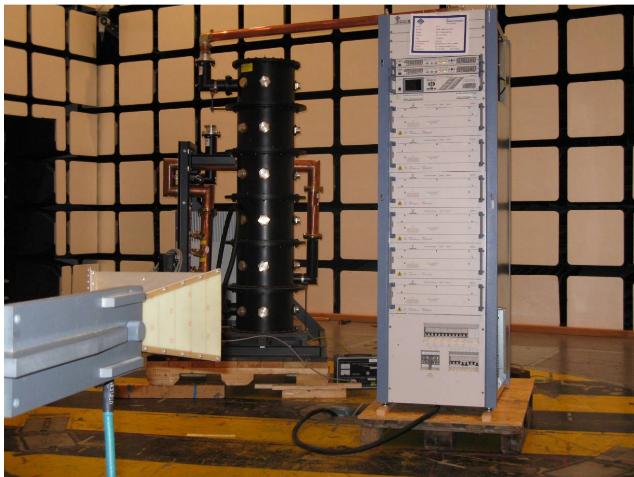
Figure 6-4: Test setup for radiated emission measurement, 1 - 10GHz
