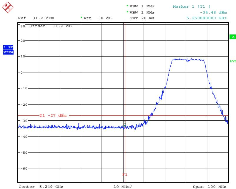
**EIRP Emission in Band on Configuration IEEE 802.11a / 5320 MHz**
