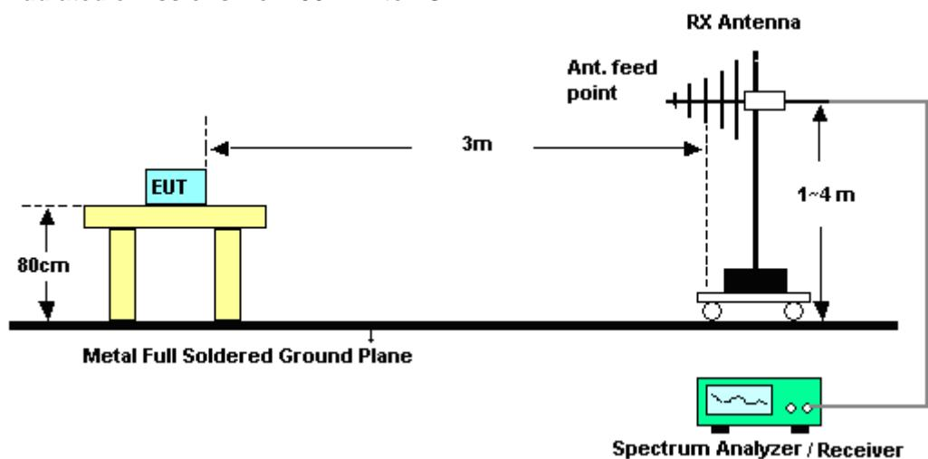
**For radiated emissions above 1GHz**
