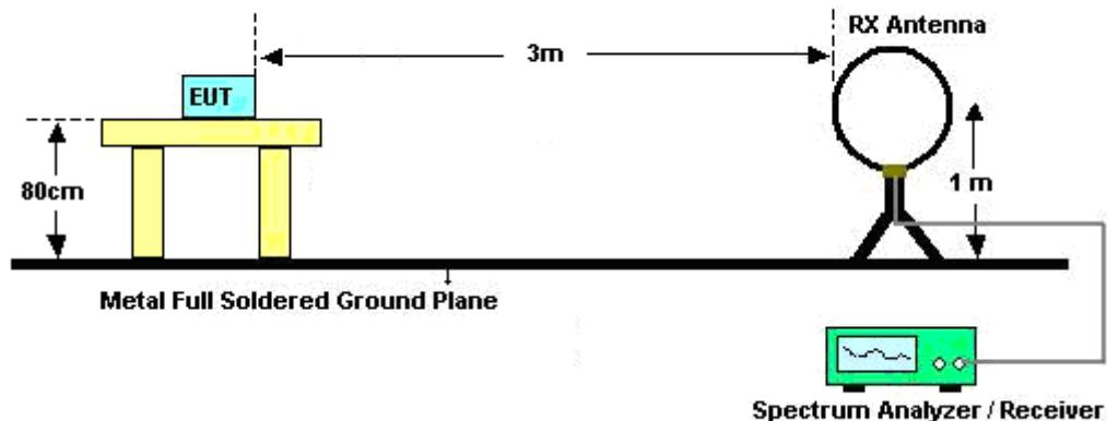
For radiated emissions from 30MHz to 1GHz
