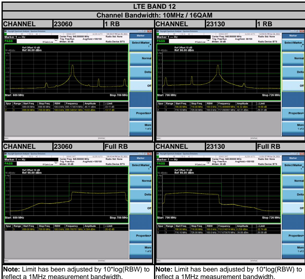
**Note:** Limit has been adjusted by  $10 \times \log(RBW)$  to reflect a 1MHz measurement bandwidth.
