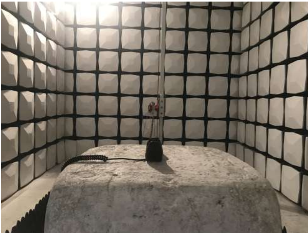
Description: Radiated Emission Test Setup for 1~18GHz
