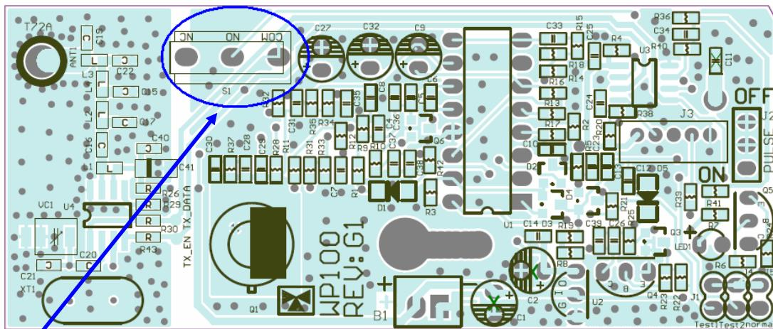
1. the angle of S1 switch rotates from 0 to 180
