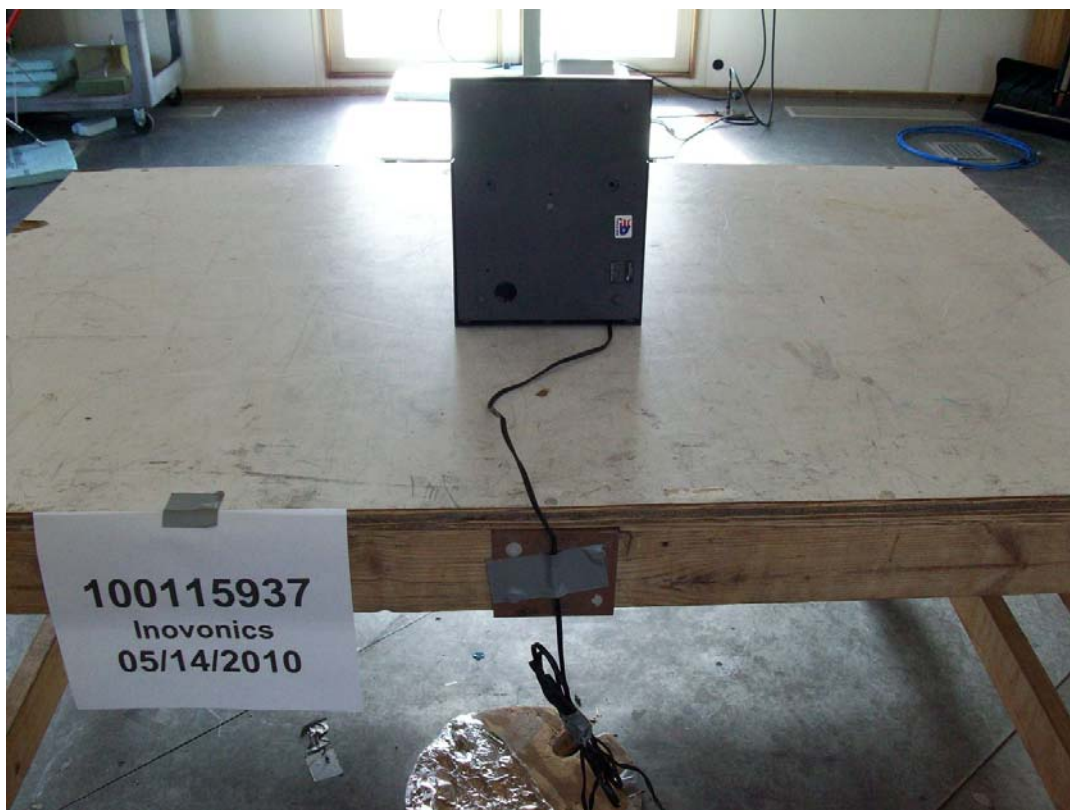
Radiated Emissions Test setup – Rear View
