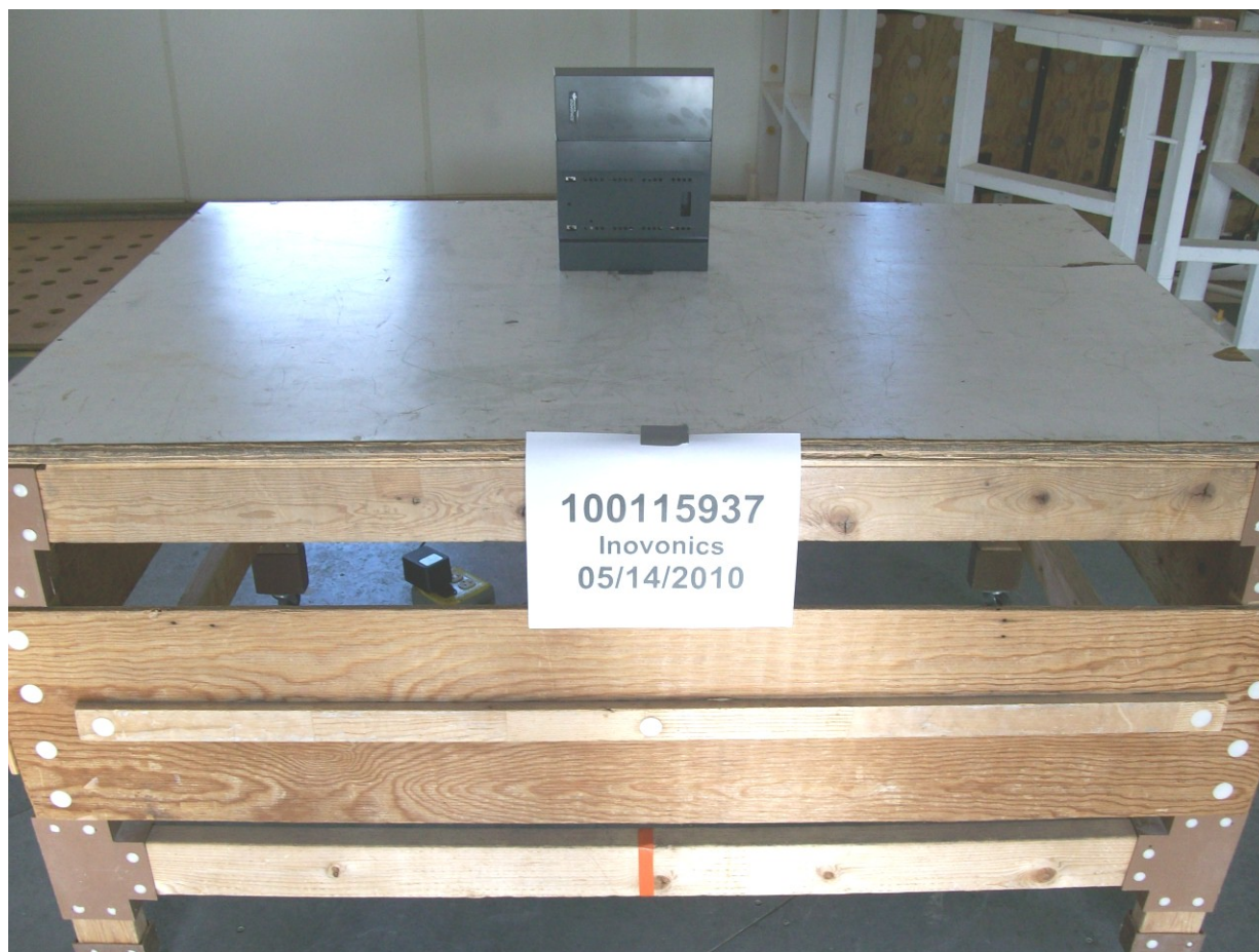
Radiated Emissions Test setup – Front View
