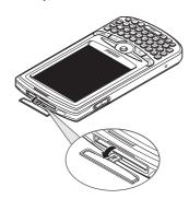
Push the card into the slot until you hear an audible system sound; this indicates that the card is already properly seated within the slot. The card is secure when it is not protruding from the base.
