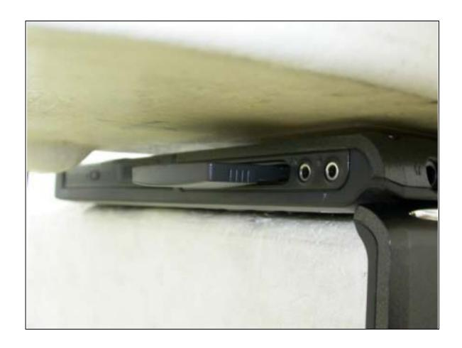
The bottom of the EUT to the phantom distance is 10mm
