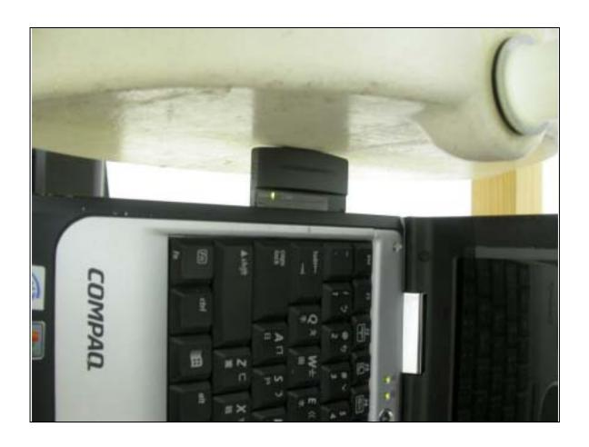
The tip of the EUT to the phantom distance is 0mm
