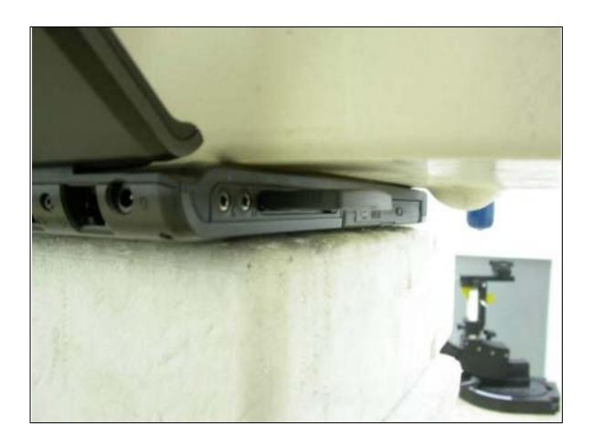
The front of the EUT to the phantom distance is 9mm
