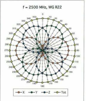
Isotropy Error ( $\phi$ ),  $\theta = 0^{\circ}$
